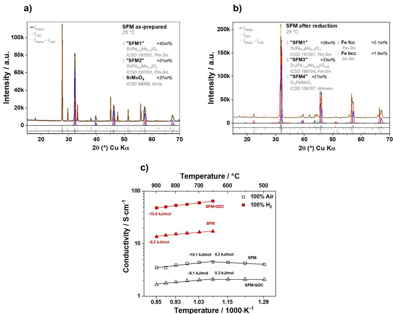
Fig. 1 Room-temperature powder XRD pattern with Rietveld refinement analysis of the as-prepared SFM in (a) air and (b) after reduction in 100% H<sub>2</sub> for 7 h at 900 °C (Rietveld data can be found in Table S1). (c) Conductivity measurements in the temperature range of 500–900 °C in air and hydrogen for SFM and the composite sample SFM-GDC. The measurements in hydrogen were conducted down to 650 °C for safety reasons.<sup>1</sup>
