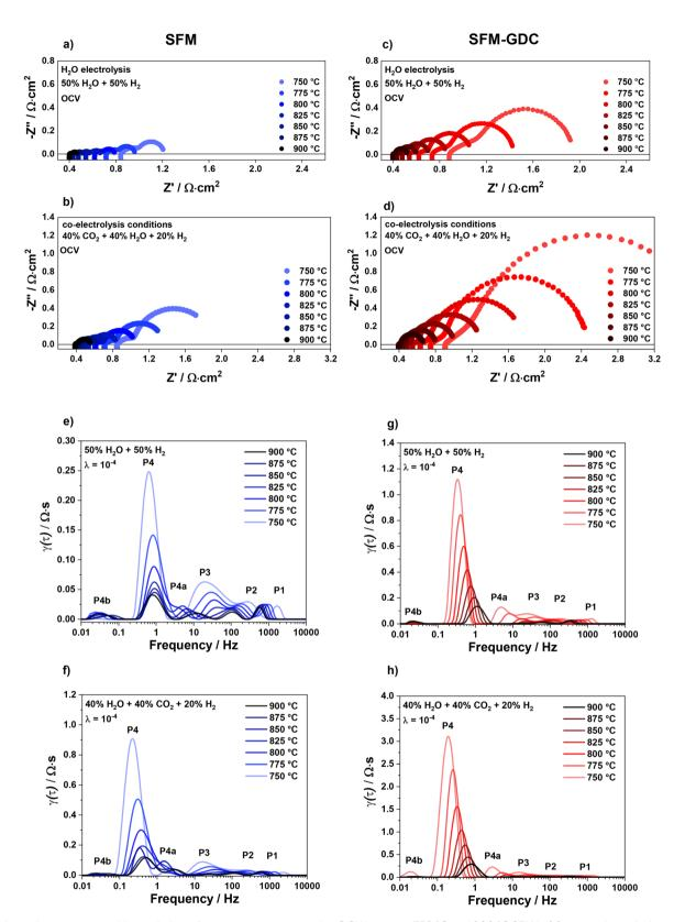
Fig. 6 Impedance spectra with a variation of temperature measured at OCV between 750 °C and 900 °C SFM in (a) steam electrolysis and (b) coelectrolysis conditions as well as SFM-GDC (c and d). In comparison, the corresponding spectra as a function of temperature for (e and f) SFM and (g and h) SFM-GDC.
