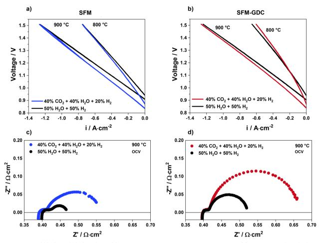
Fig. 5 I-V curves at 800 °C and 900 °C for SFM in (a) steam electrolysis and co-electrolysis compared to (b) the composite SFM-GDC in steam electrolysis and co-electrolysis conditions. The corresponding impedance spectra at 900 °C recorded in steam electrolysis and co-electrolysis are given for (c) SFM and (d) the SFM-GDC composite.
