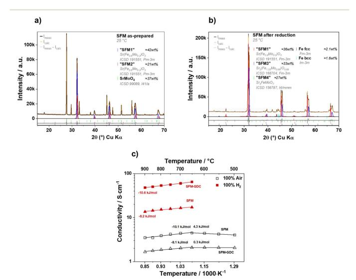
Fig. 1 Room-temperature powder XRD pattern with Rietveld refinement analysis of the as-prepared SFM in (a) air and (b) after reduction in 100%  $H_2$  for 7 h at 900 °C (Rietveld data can be found in Table S1). (c) Conductivity measurements in the temperature range of 500–900 °C in air and hydrogen for SFM and the composite sample SFM-GDC. The measurements in hydrogen were conducted down to 650 °C for safety reasons.<sup>1</sup>
