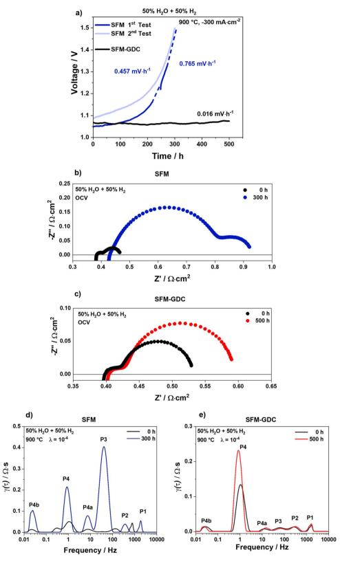
Fig. 8 (a) Long-term stability test of single cells with SFM/GDC/8YSZ/GDC/LSCF and the composite SFM-GDC/GDC/8YSZ/GDC/LSCF in 50% H<sub>2</sub>O + 50% H<sub>2</sub> fuel gas composition under constant -0.3 A cm<sup>-2</sup> current load at 900 °C for up to 500 h. Comparison of (b and c) the Nyquist plots and (d and e) the corresponding DRT spectra recorded before and after the durability test.
