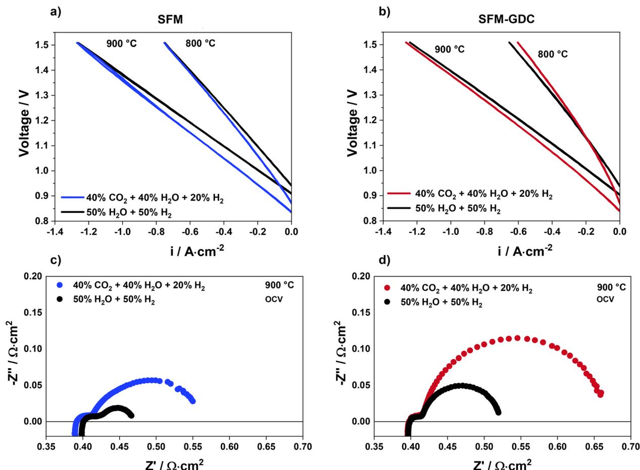
Fig. 5  $I$ - $V$  curves at 800 °C and 900 °C for SFM in (a) steam electrolysis and co-electrolysis compared to (b) the composite SFM-GDC in steam electrolysis and co-electrolysis conditions. The corresponding impedance spectra at 900 °C recorded in steam electrolysis and co-electrolysis are given for (c) SFM and (d) the SFM-GDC composite.
