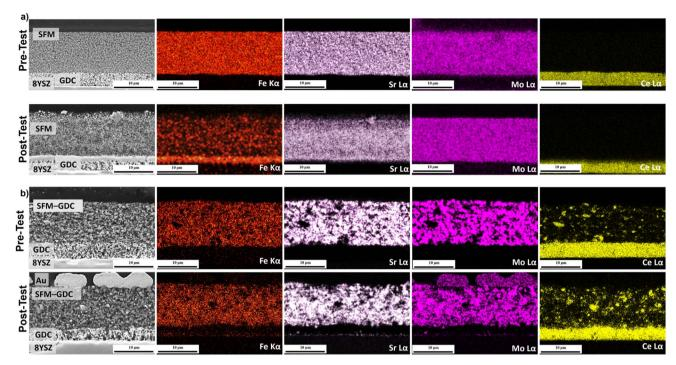
Fig. 9 Cross-sectional SEM-EDX mapping of the fuel electrode side for Sr (Lα, 13.89 keV). Fe (Kα, 6.40 keV). Mo (Lα, 17.14 keV). Ce (Lα, 33.90 keV) lines of as-prepare and tested (a) SFM and (b) SFM-GDC single cells operating in steam electrolysis at -0.3 A cm<sup>-2</sup> up to 500 h.
