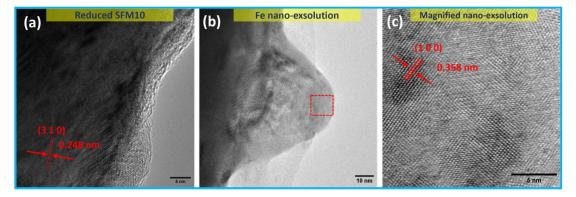
Fig. 4 (a) HRTEM image of reduced SFM, TEM image of (b) reduced SFM with exsolution illustrating the anchoring effect of the Fe nanoexsolution with the SFM matrix, (c) HRTEM image of Fe nano-exsolution of the inset marked with red box depicted in (b).
