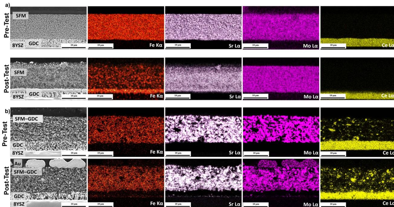
Fig. 9 Cross-sectional SEM-EDX mapping of the fuel electrode side for Sr ( $L\alpha$ , 13.89 keV), Fe ( $K\alpha$ , 6.40 keV), Mo ( $L\alpha$ , 17.14 keV), Ce ( $L\alpha$ , 33.90 keV) lines of as-prepare and tested (a) SFM and (b) SFM-GDC single cells operating in steam electrolysis at  $-0.3 \text{ A cm}^{-2}$  up to 500 h.
