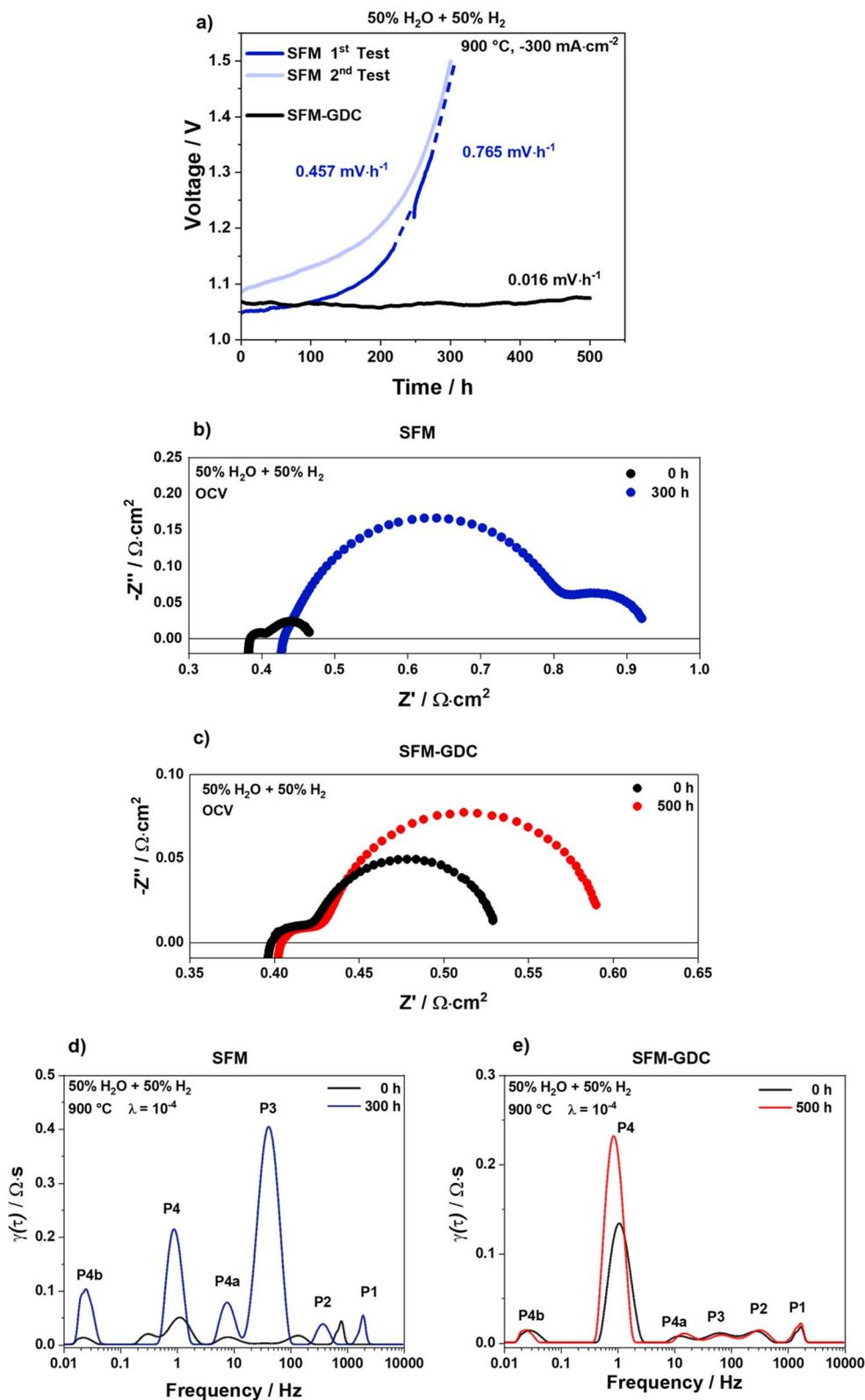
Fig. 8 (a) Long-term stability test of single cells with SFM/GDC/8YSZ/GDC/LSCF and the composite SFM-GDC/GDC/8YSZ/GDC/LSCF in 50% H<sub>2</sub>O + 50% H<sub>2</sub> fuel gas composition under constant  $-0.3 \text{ A cm}^{-2}$  current load at 900 °C for up to 500 h. Comparison of (b and c) the Nyquist plots and (d and e) the corresponding DRT spectra recorded before and after the durability test.
