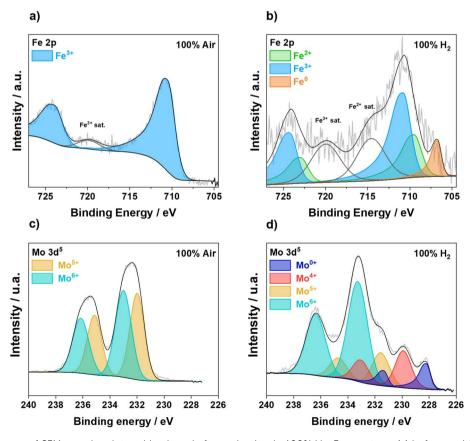
Fig. 2 Selected XPS scans of SFM samples sintered in air and after reduction in 100% H<sub>2</sub>. Fe spectrum (a) before and (b) after reduction. Mo spectrum (c) before and (d) after reduction.
