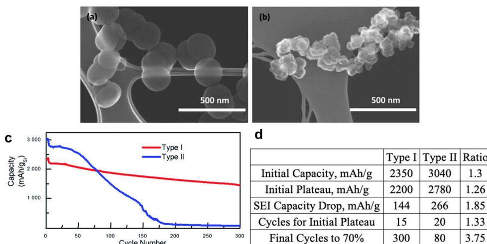
Fig. 9 TEM micrographs of silicon particles showing (a) Type I and (b) Type II particles and (c) associated capacity versus cycle number.<sup>54</sup> (d) A summary of the capacity of batteries for type I and type II particles versus cycle number. First three cycles are at C/20, while the remaining are at C/10. Table shows values for some of the features in the plot.
