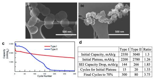
Fig. 9 TEM micrographs of silicon particles showing (a) Type I and (b) Type II particles and (c) associated capacity versus cycle number. 54 (d) A summary of the capacity of batteries for type I and type II particles versus cycle number. First three cycles are at C/20, while the remaining are at C/10. Table shows values for some of the features in the plot.
