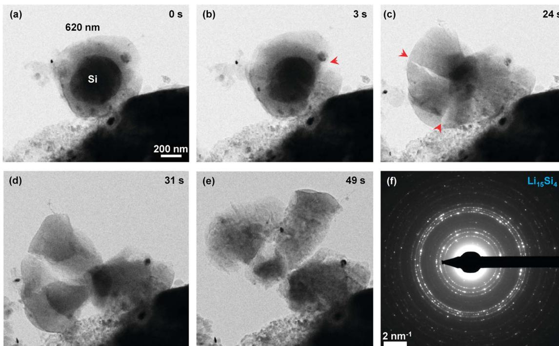
Fig. 2 (a–e) Lithiation of a 620 nm crystalline silicon particle with deprecation. Red arrows indicate cracks. (f) Electron diffraction indicating the formation of polycrystalline  $\text{Li}_{15}\text{Si}_4$  upon lithiation. Images reproduced from ref. 10.
