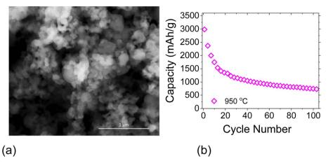
Fig. 10 Bioinspired silica, reduced at 950 °C; (a) SEM micrograph and (b) capacity versus cycle number, image reproduced with permission from ref. 27.
