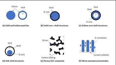
Fig. 4 Strategies to engineer the particle microstructure (left) and morphology to prevent breakage (decrepitation), right. Images reproduced from ref. 15 and 19
