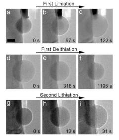
Fig. 5 Lithiation and delithiation of Si nanoparticles (the scale bar = 200 nm): first lithiation cycle (a-c), first delithiation (d-f), and second lithiation (g-i). Images reproduced from ref. 7.
