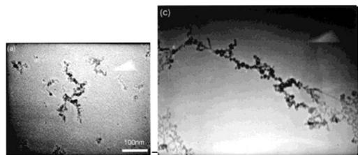
Fig. 6 Deformation of titania aggregates in TEM by >200% (from the image on left to the image on right). Image reproduced with permission from ref. 38.
