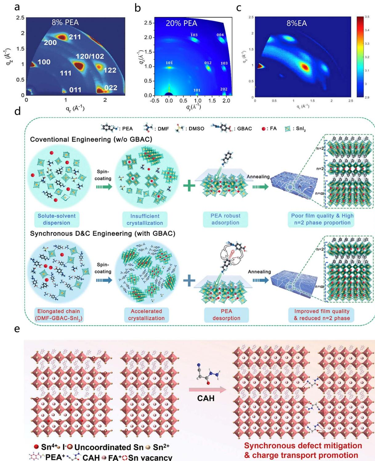
Fig. 11 GIWAXS of (a) 8% PEA, (b) 20% PEA, and (c) 8% EA.<sup>85</sup> Copyright 2017, Wiley-VCH GmbH. (d) Schematic of the action mechanism of GBAC.<sup>115</sup> Copyright 2025, the Royal Society of Chemistry. (e) Schematic of the interaction between CAH and Sn perovskite.<sup>117</sup> Copyright 2025, Wiley-VCH GmbH.
