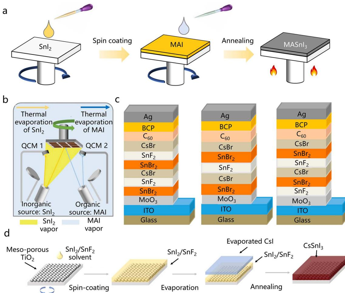
Fig. 4 (a) Procedure of the spin-coating method (using the two-step method as an example). (b) Procedure of the thermal co-evaporation method.<sup>70</sup> Copyright 2023, the American Chemical Society. (c) Example of the sequential co-evaporation method.<sup>71</sup> Copyright 2023, Wiley-VCH GmbH. (d) Procedure of the VASP method.<sup>74</sup> Copyright 2023, Wiley-VCH GmbH.
