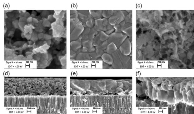
Fig. 4 Top-view (a) TF-1, (b) TF-2, and (c) TF-3, and cross-sectional view (d) TF-1, (e) TF-2, and (f) TF-3. SEM images of the CZTS thin film (TF) annealed at 650 °C for 20 min.
