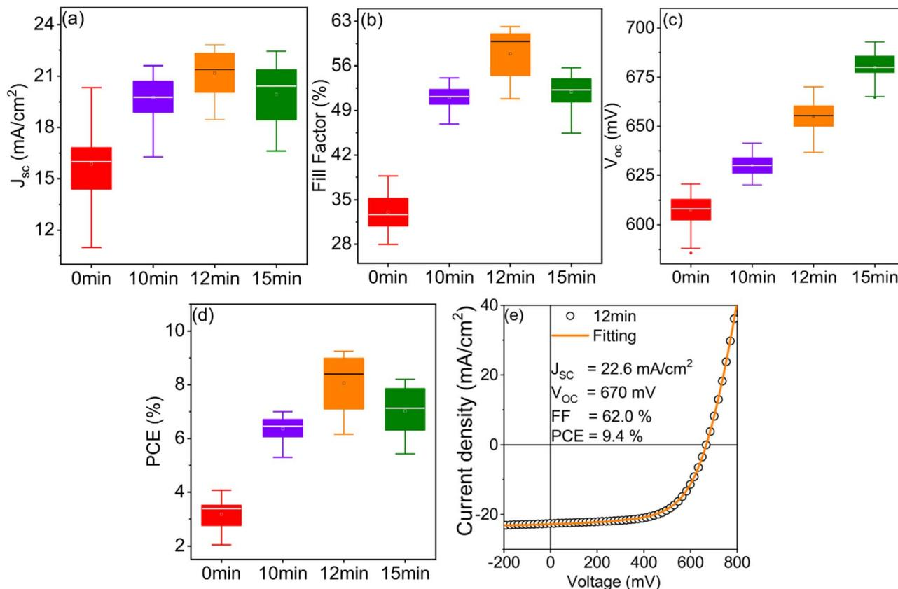
Fig. 7 Plots of solar cell output parameters: (a)  $J_{SC}$ , (b) FF, (c)  $V_{OC}$ , and (d) PCE for SC2 device subjected to different post-annealing durations of the complete glass/Mo/CZTS/CdS/i-ZnO/ITO structure (SC2-0 min, SC2-10 min, SC2-12 min, and SC2-15 min); (e)  $J$ - $V$  curve of the champion device with corresponding fitting result using eqn (9).
