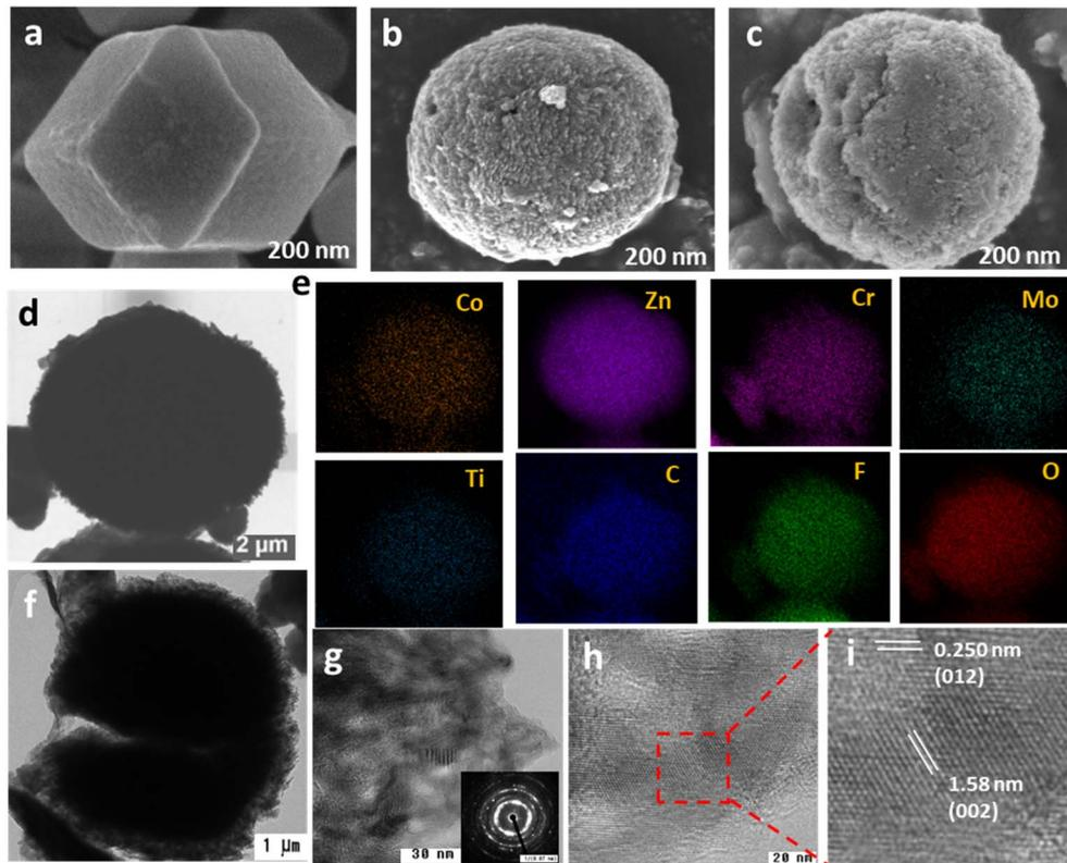
Fig. 2 SEM image of as-prepared (a) ZIF-67, (b) CoZnCr and (c) CoZnCr@Mo<sub>2</sub>TiC<sub>2</sub>. (d) STEM image of as prepared CoZnCr@Mo<sub>2</sub>TiC<sub>2</sub>. (e) Elemental mapping showing the uniform distribution of Co, Zn, Cr, Mo, Ti and C. (f and g) HRTEM image of CoZnCr@Mo<sub>2</sub>TiC<sub>2</sub>. (h and i) Lattice fringes of CoZnCr and Mo<sub>2</sub>TiC<sub>2</sub>.
