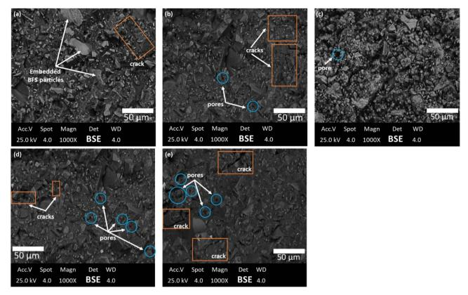
Fig. 7 Backscattered electron image of (a) AAM<sub>1.5, 0.4, 3.0</sub>, (b) AAM<sub>1.0, 0.4, 3.0</sub>, (c) AAM<sub>0.5, 0.4, 3.0</sub>, (d) AAM<sub>0.5, 0.4, 2.5</sub>, and (e) AAM<sub>0.5, 0.4, 2.6</sub>
