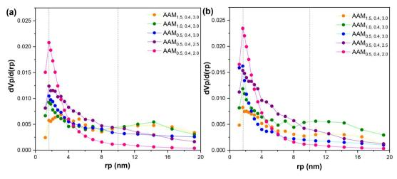
Fig. 9 PSD curves of AAMs after (a) 7 and (b) 28 days
