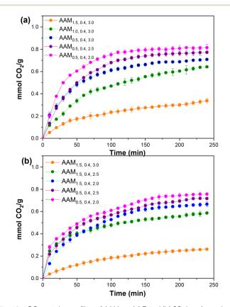
Fig. 10  $\,$  CO $_2$  uptake profiles of AAMs at (a) 7 and (b) 28 days (error bars are standard errors).
