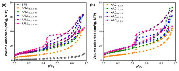
Fig. 8 Nitrogen adsorption—desorption isotherms of AAMs at (a) 7 and (b) 28 days.
