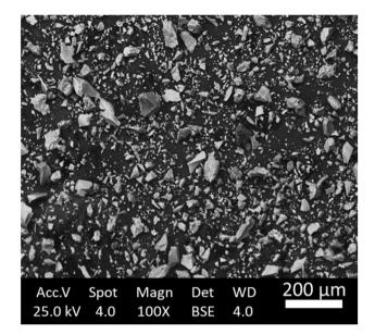
Fig. 5 Backscattered electron image of BFS.
