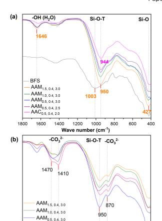
Fig. 11 FTIR spectra of BFS and AAMs (a) before and (b) after  $\rm CO_2$  uptake.
