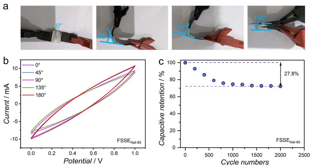
Fig. 6 (a) Digital photographs of an all-solid-state supercapacitor under bending at different angles of 0°, 45°, 90°, and 180°. (b) Cyclic voltammetry curves at 100 mV s<sup>-1</sup>. (c) Cycling stability test at a current density of 5 A g<sup>-1</sup> under 90° bending conditions.
