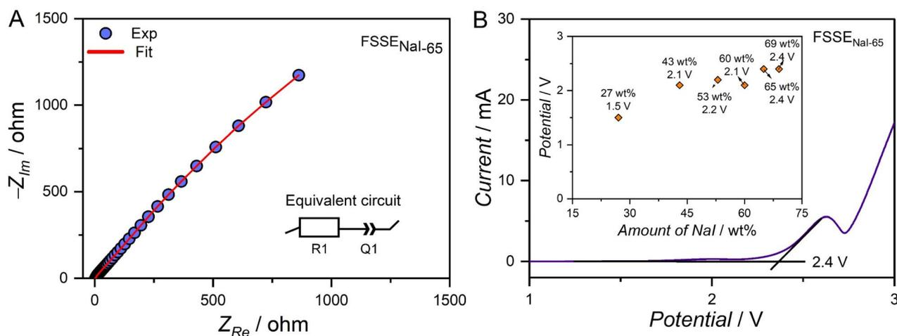
Fig. 4 (a) Nyquist plot of FSSE<sub>NaI-65</sub>.  $Z_{Re}$  and  $Z_{Im}$  are the real and imaginary components, respectively. The red line indicates the fitting of impedance data by using the specified equivalent circuit. (b) Linear sweep voltammetry (LSV) measurement for FSSE<sub>NaI-65</sub>. (Inset): trends of LSV with the variation of NaI content from 27 wt% to 69 wt%.
