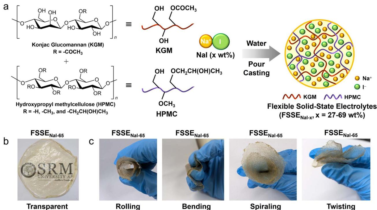
Fig. 1 (a) Schematic representation for the preparation of flexible solid-state electrolytes (FSSE<sub>NaI-x</sub>, x = 27–69 wt%). (b) An image of a representative transparent film of FSSE<sub>NaI-65</sub>. (c) Photographs of various modes of flexibility of a representative FSSE<sub>NaI-65</sub> film.
