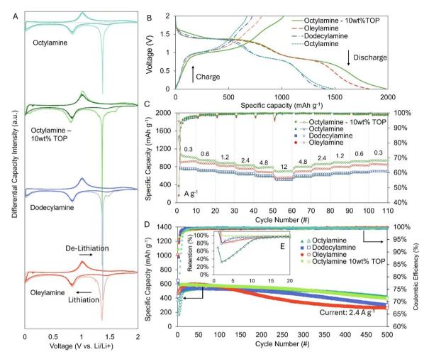
Fig. 6 Li-ion electrochemical data of the ultrasmall  $Sb_2S_3$  synthesized in different ligating environments. (A) Total differential capacity data of the first (lighter) and second (darker) cycle for nanoparticles synthesized using identified alkylamine. (B) Galvanostatic charge—discharge curves of the first cycle. (C) Rate capacity. (D) Cycling stability data. (E) Normalized cycling stability data of the first 20 cycles.
