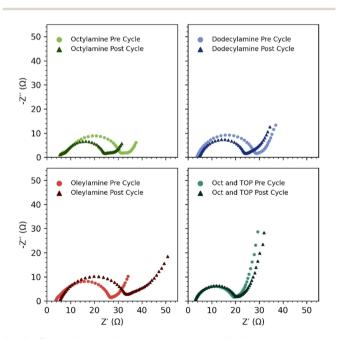
Fig. 7 Electrochemical impedance spectra of electrodes prepared with  $\mathrm{Sb}_2\mathrm{S}_3$  nanoparticles synthesized using octylamine (oct), dode-cylamine, oleylamine, and octylamine with trioctylphosphine (TOP) before and after cycling 20 times at 2.4 A g<sup>-1</sup>.
