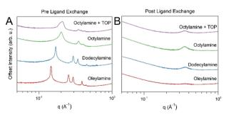
Fig. 5 SAXS spectra of (A)  $\mathrm{Sb}_2\mathrm{S}_3$  particles before ligand exchange synthesized with oleylamine, dodecylamine, octylamine, as well as octylamine with 10 wt% trioctylphosphine (TOP). (B) After synthesizing, the particles were washed and ligand exchanged with hydrazine (procedure in methods) before being dispersed in water and characterized in SAXS. Both axes in log scale.
