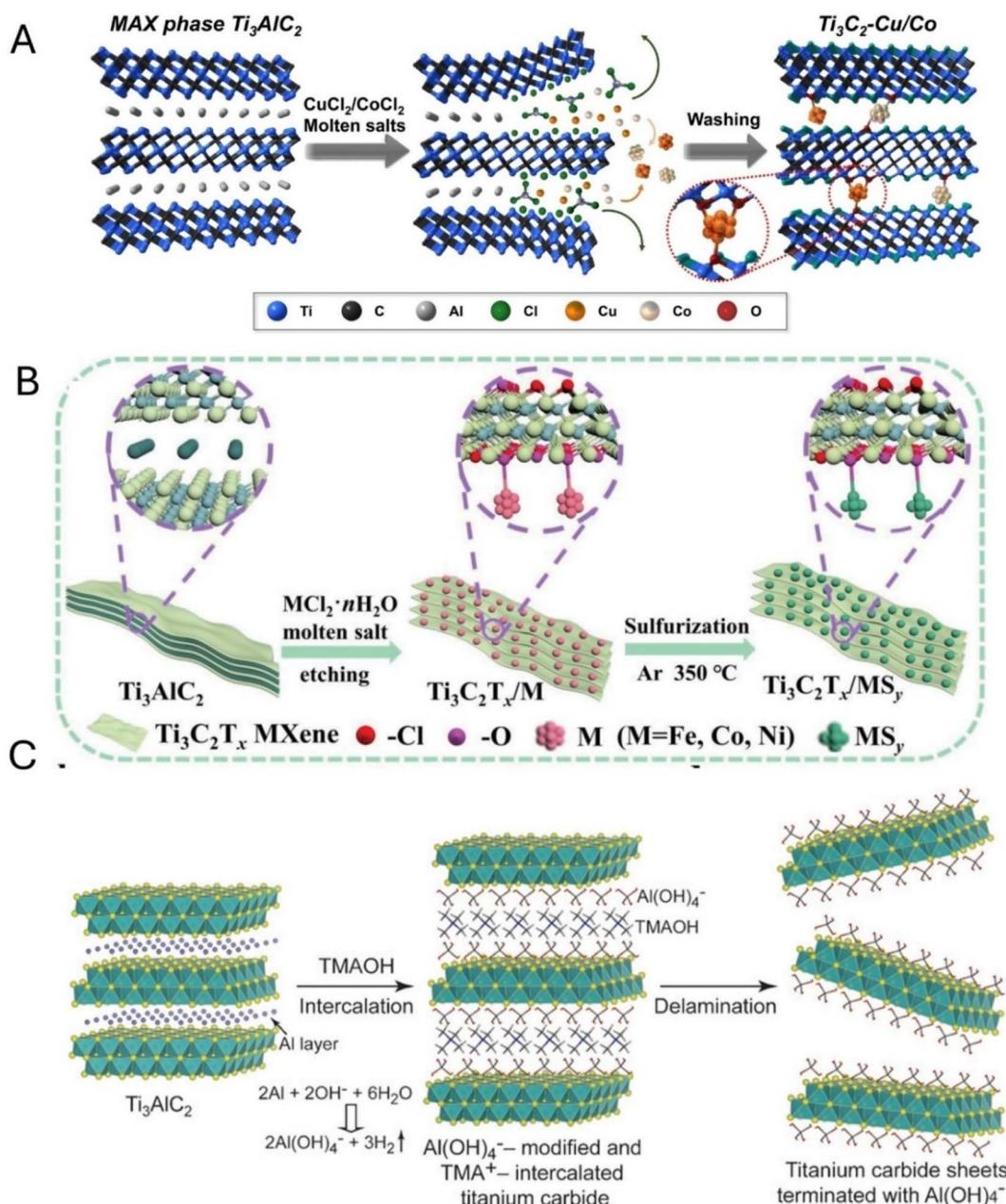
Fig. 5 (A) Schematic illustration of MXene hybrid formulation of  $Ti_3C_2-Cu/Co$ . Reproduced with permission.<sup>168</sup> Copyright 2021 Wiley-VCH. (B) A graphic visual of the fabrication procedure of the  $Ti_3C_2T_x/MS_y$  heterostructures. Reproduced with permission.<sup>169</sup> Copyright 2022, Wiley-VCH. (C) Graphic demonstration of the intercalation and delamination method for MXene using TMAOH. Reproduced with permission.<sup>129</sup> Copyright 2016, Wiley-VCH.
