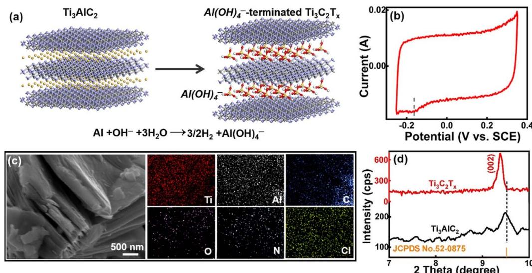
Fig. 10 (a) Schematic illustration of the fabrication process and morphological structure of the fluoride-free electrochemical etched MXene  $\text{Ti}_3\text{C}_2\text{T}_x$ . (b) The three-electrode configuration was employed to acquire the CV scan for the MAX electrode with a scan rate of  $20 \text{ mV s}^{-1}$ . (c) SEM and elemental mapping analysis images, and (d) XRD patterns of MXene and MAX phase. Reproduced with permission.<sup>204</sup> Copyright 2023, American Chemical Society.
