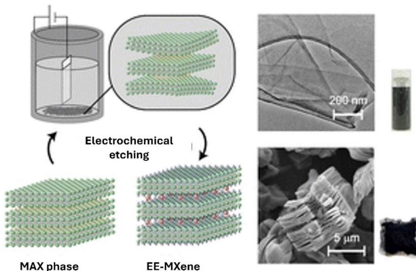
**Fig. 11** Schematic illustration of the low-fluoride electrochemical etching fabrication of MXene along with the TEM micrograph of delaminated MXene and SEM micrographs of MXene powder. Reproduced with permission.<sup>145</sup> Copyright 2024, The Royal Society of Chemistry under Creative Commons Attribution 3.0 Unported License.
