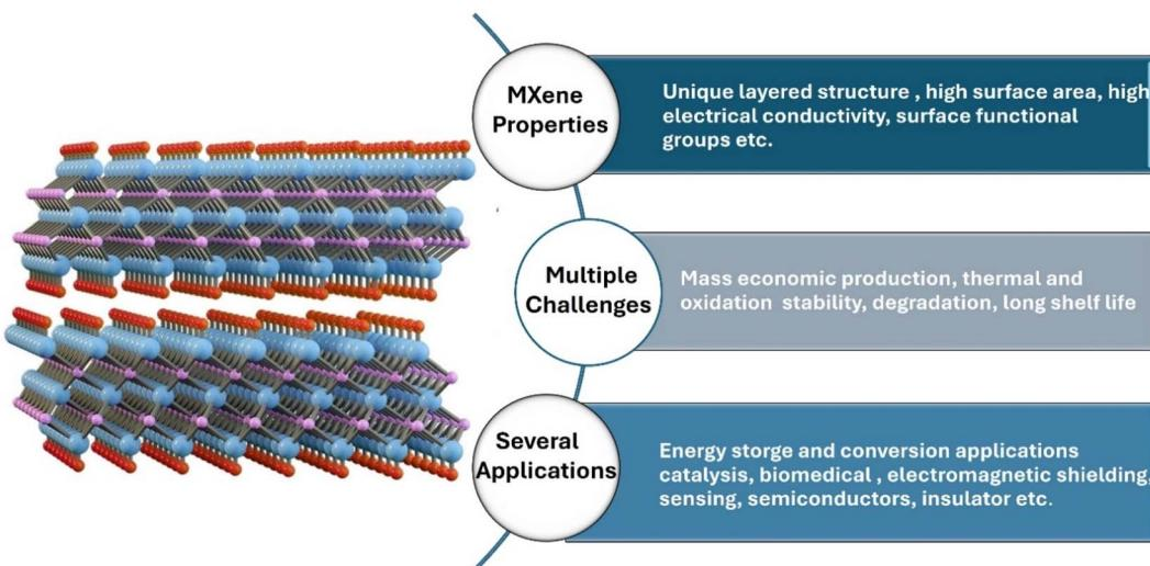
Fig. 1 The MXene properties, multiple applications and wide-ranging applications. MXene structure. Reproduced with permission.<sup>172</sup> Copyright 2021, Wiley-VCH.
