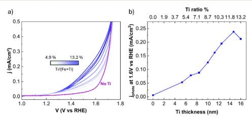
Fig. 2 (a) Linear sweep voltammetries under UV illumination for the Ti:Fe<sub>2</sub>O<sub>3</sub> $|\Delta$ Ti sample: the one on the point with no titanium is coloured in purple. (b) Photocurrents at 1.6 V vs. RHE at different Ti content for the sample: the photocurrents have been computed subtracting the value of current for the LSV in the dark at that potential from the one under illumination.
