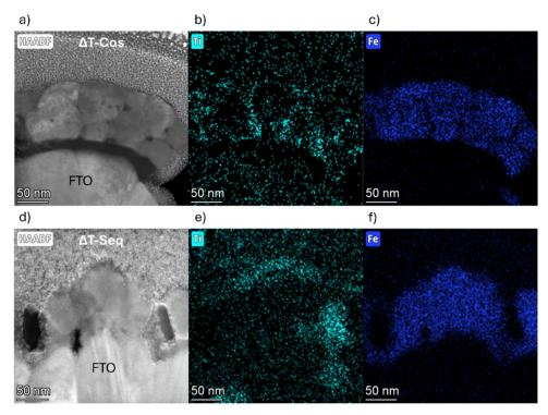
Fig. 7 TEM images and elemental maps. (a) image, (b) Ti and (c) Fe elemental maps for the point at 750 °C on Ti:Fe<sub>2</sub>O<sub>3</sub>| $\Delta T$ -cos; (d) image, (e) Ti and (f) Fe elemental maps for a point at 750 °C on Ti: $Fe_2O_3|\Delta T$ -seq.
