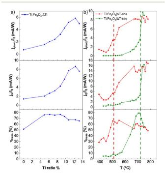
Fig. 4 Normalized photocurrent (upper frames), normalized  $j_G$  (central frames) and transfer efficiency (lower frames) obtained by fitting IMPS data acquired at  $1.45\,\mathrm{V}$  vs. RHE with a DRT algorithm for (a) Ti:Fe<sub>2</sub>O<sub>3</sub>| $\Delta T$ , (b) Ti:Fe<sub>2</sub>O<sub>3</sub>| $\Delta T$ -cos and Ti:Fe<sub>2</sub>O<sub>3</sub>| $\Delta T$ -seq. The lines mark the points of highest derivative for the photocurrents.
