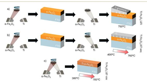
Fig. 1 Schematic depiction of the fabrication steps for the three different kinds of samples analysed in the study: (a) Ti:Fe<sub>2</sub>O<sub>3</sub>| $\Delta$ Ti; (b) Ti:Fe<sub>2</sub>O<sub>3</sub>| $\Delta$ T-seq and (c) Ti:Fe<sub>2</sub>O<sub>3</sub>| $\Delta$ T-cos.
