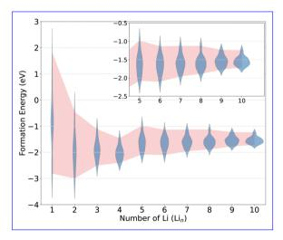
Fig. 7 Progression in formation energy as a function of number of Li in the range Li $_1$  to L $_{10}$ . For each concentration, the violin plot shows the underlying distribution resulting from the structural ensemble. The red envelope function provides a guide for the eye. The inset zooms into the concentration range from Li $_5$  to Li $_{10}$ .
