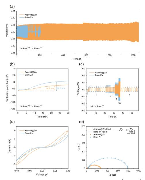
Fig. 4 (a) Long cycling performance and (b) nucleation overpotentials of the Zn symmetric cells at 1 mA cm $^{-2}$ , 1 mAh cm $^{-2}$ . (c) Rate performance of the Zn symmetric cells at a capacity of 1 mAh cm $^{-2}$ . (d) Cyclic voltammetry (CV) curves of the Zn symmetric cells measured at 1 mV s $^{-2}$ . (e) EIS plots of the symmetric cells before cycling.
