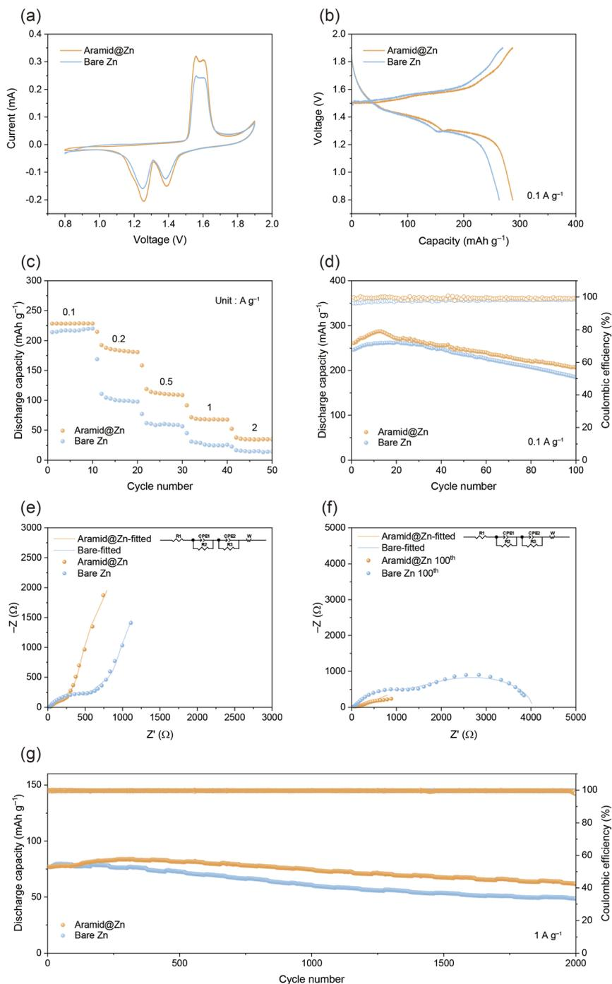
Fig. 5 Zn|| $\alpha$ -MnO<sub>2</sub> full cells with Bare Zn and Aramid@Zn anodes. (a) CV curves at a scan rate of 0.1 mV s<sup>-1</sup>. (b) Galvanostatic charge-discharge curves at 0.1 A g<sup>-1</sup>. (c) Rate performance at current densities ranging from 0.1 to 2 A g<sup>-1</sup>. (d) Cycling performance at 0.1 A g<sup>-1</sup>. (e) EIS plots of the full cells before cycling and (f) after 100 cycles. (g) Cycling performance at 1 A g<sup>-1</sup>.
