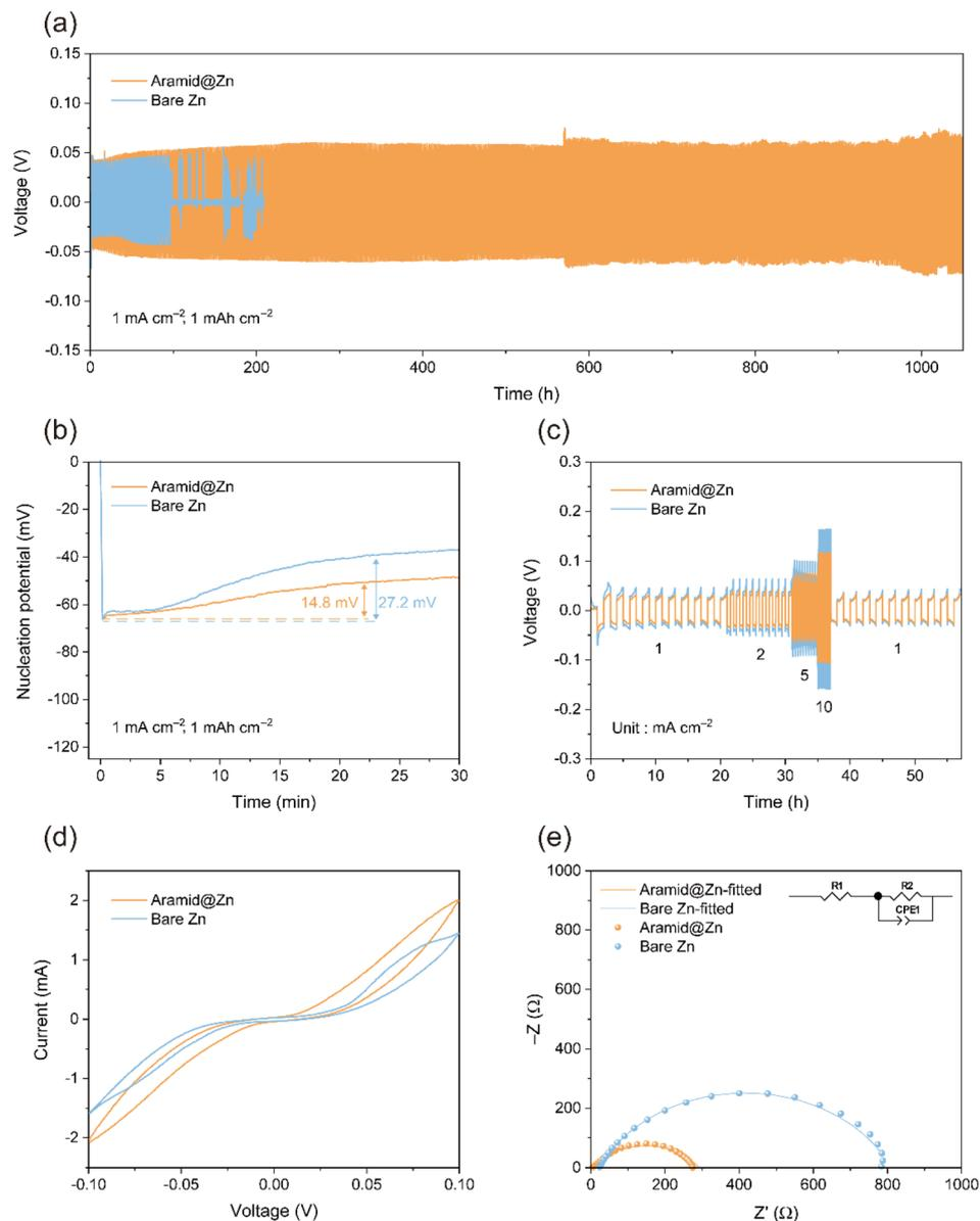
Fig. 4 (a) Long cycling performance and (b) nucleation overpotentials of the Zn symmetric cells at  $1 \text{ mA cm}^{-2}$ ,  $1 \text{ mAh cm}^{-2}$ . (c) Rate performance of the Zn symmetric cells at a capacity of  $1 \text{ mAh cm}^{-2}$ . (d) Cyclic voltammety (CV) curves of the Zn symmetric cells measured at  $1 \text{ mV s}^{-2}$ . (e) EIS plots of the symmetric cells before cycling.
