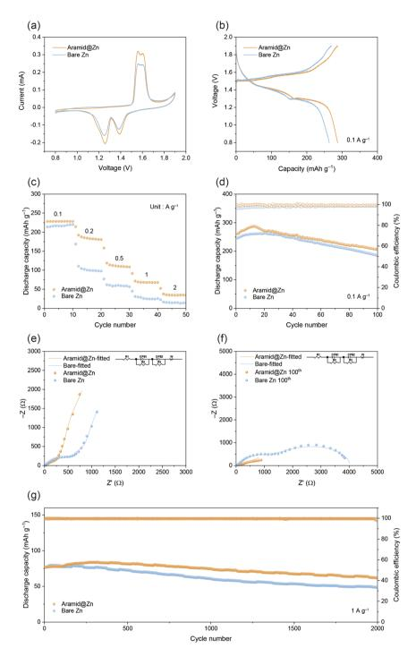
Fig. 5  $Zn\|\alpha-MnO_2$  full cells with Bare Zn and Aramid@Zn anodes. (a) CV curves at a scan rate of 0.1 mV s<sup>-1</sup>. (b) Galvanostatic charge–discharge curves at 0.1 A g<sup>-1</sup>. (c) Rate performance at current densities ranging from 0.1 to 2 A g<sup>-1</sup>. (d) Cycling performance at 0.1 A g<sup>-1</sup>. (e) EIS plots of the full cells before cycling and (f) after 100 cycles. (g) Cycling performance at 1 A g<sup>-1</sup>.
