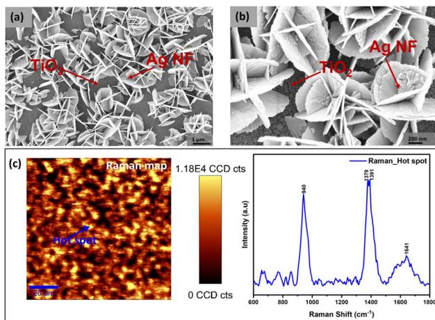
Fig. 1 SEM image of Ag NFs on TiO<sub>2</sub> thin film at (a) low magnification and (b) high magnification. (c) Raman map of Ag NFs with corresponding normal Raman spectra of the Ag–TiO<sub>2</sub> hot spot region.
