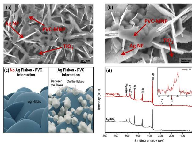
Fig. 2 SEM image of PVC-MNPs loaded on Ag–TiO<sub>2</sub> thin film at (a) low magnification and (b) high magnification. (c) Schematic depiction of the interaction of PVC-MNPs with Ag NFs, and (d) XPS analysis of pristine Ag–TiO<sub>2</sub> and Ag–TiO<sub>2</sub> loaded with PVC-MNPs with insets of Cl 2p.
