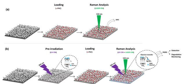
Fig. 3 Schematic of (a) SERS detection of PVC-MNPs on Ag-TiO<sub>2</sub> platform and (b) PIERS detection and degradation monitoring of PVC-MNPs on Ag-TiO<sub>2</sub> platform. For each PIERS signal acquisition during Raman analysis, laser ( $\lambda = 532$  nm with 40 mW of power) was on for only 30 s and for degradation monitoring of PVC-MNPs, PIERS signals were acquired at cumulative time intervals of 10 min, 20 min, and 30 min of UV on.
