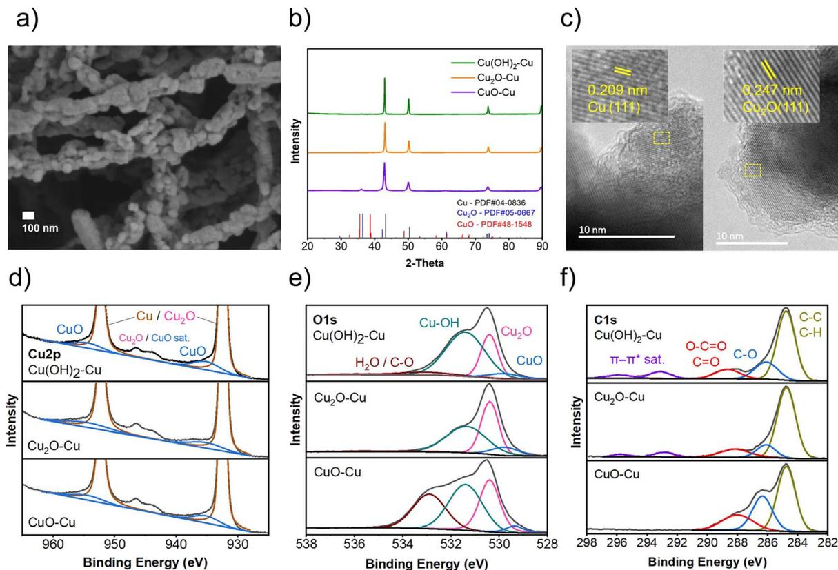
Fig. 2 Characterization of the Cu electrocatalysts. (a) SEM image of CuO-Cu, (b) XRD patterns of Cu(OH)<sub>2</sub>-Cu, Cu<sub>2</sub>O-Cu, and CuO-Cu electrocatalysts. (c) TEM images of CuO-Cu. (d) Cu 2p, (e) O 1s, and (f) C 1s XPS peak-fitting results of the three electrocatalysts. CuO-Cu reveals an exceptionally high O 1s peak at 532.9 eV.
