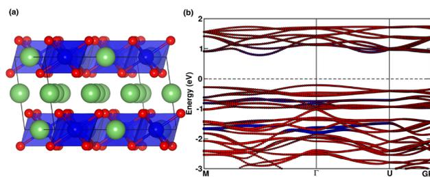
Fig. 1 (a) Crystal structure of  $\text{Li}_2\text{NiO}_3$  in pristine state and (b) the corresponding non-magnetic DFT band structure. The representative colors for the fat bands as well as the atomic spheres are Ni (blue), O (red), and Li (green). The Fermi energy is marked with the dashed line at 0 eV.
