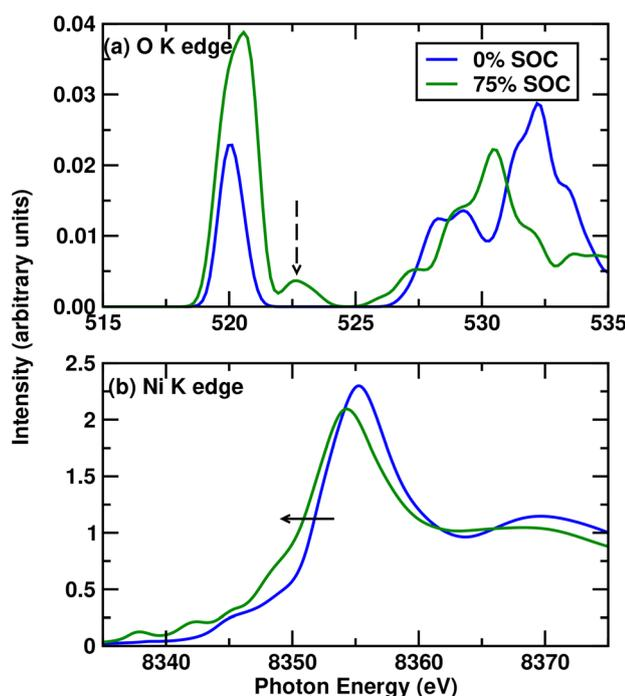
Fig. 4 Figure showing (a) O–K and (b) Ni K edges for  $\text{Li}_2\text{NiO}_3$  at the beginning and near the end of charge at 0% and 75% SOC. The dashed arrow in (a) indicates the peak generally shown in experimental studies to indicate the O dimer, while the solid arrow in (b) shows the movement of the Ni K edge as a function of state of charge.
