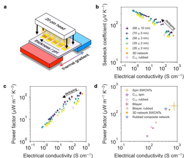
**Fig. 4** (a) High-throughput setup used to measure  $\sigma$  and *S* of up to five samples in parallel across a thermal gradient established in between two Peltier modules. (b) *S* and (c) PF as a function of  $\sigma$  of F4TCNQ-doped and (thermally) dedoped rubbed networks of SWCNTs and PBTTC-C<sub>12</sub>. (d) Highest TE PFs obtained among the F4TCNQ-doped samples.
