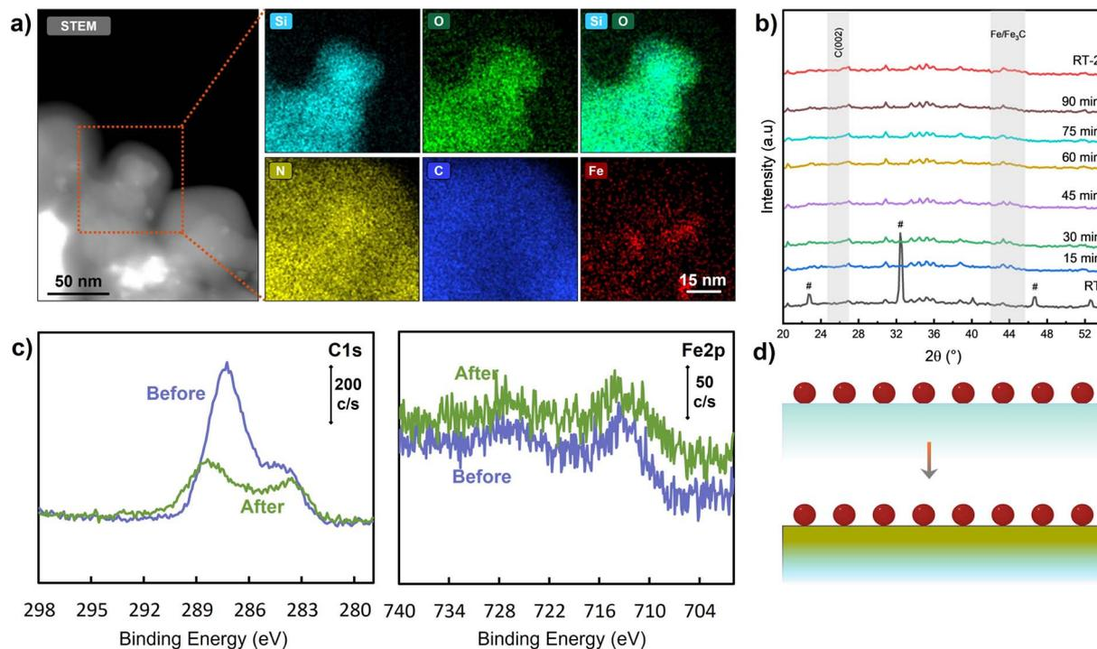
Fig. 5 (a) STEM-EDS, (b) *in situ* XRD, (c) C1s and Fe 2p XPS and (d) schematic representation of Fe/Si<sub>3</sub>N<sub>4</sub> after reaction.
