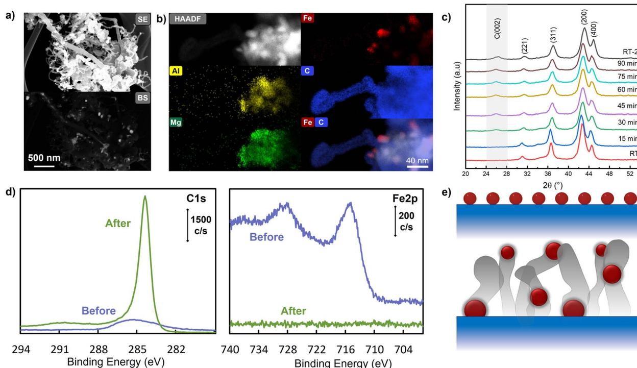
Fig. 7 (a) SEM, (b) *in situ* XRD, (c) C1s and Fe 2p XPS and (d) schematic representation of Fe/MgAlO<sub>x</sub> after reaction.
