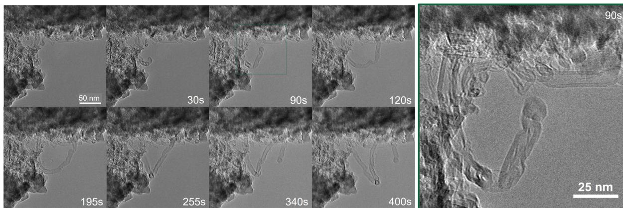
Fig. 9 Beam-enhanced *in situ* TEM of FeNPs supported on MgAl<sub>2</sub>O<sub>4</sub>. Time frame indicated in seconds.
