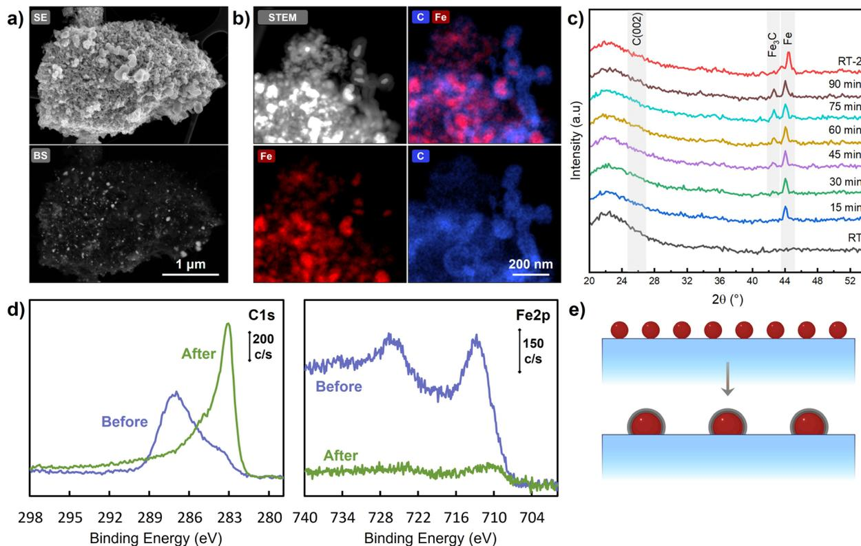
Fig. 3 (a) SEM, (b) STEM-EDS, (c) *in situ* XRD, (d) C1s and Fe 2p XPS and (e) schematic representation of Fe/SiO<sub>2</sub> after reaction.
