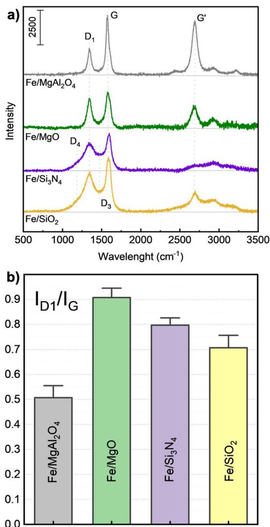
Fig. 8 (a) Raman spectra and (b)  $I_{\text{D}_1}/I_{\text{G}}$  values of spent catalysts.
