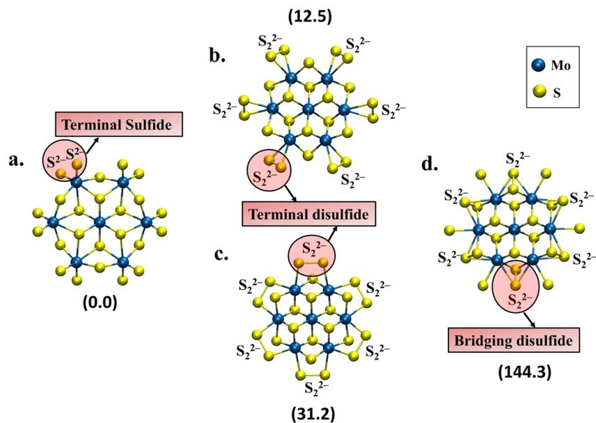
Fig. 3 (a–d) Possible structures considered for modeling the sulfided analog of Anderson polyoxometalate  $[\text{Mo}^{\text{VI}}_7\text{O}_{24}]^{6-}$  and their relative Gibbs free energies (in parentheses) at standard state in units of  $\text{kcal mol}^{-1}$ . Structures a, b, c, and d have the same labels as in the text.
