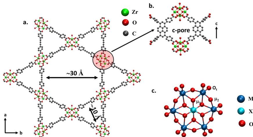
Fig. 1 (a) Crystal structure of NU-1000, showing 30 and 10 Å channels along the *c*-axis, (b) side view of the *c* pore, (c) top views of an  $\alpha$ -type planar Anderson POM, which can be anchored in the *c* pore. X represents a heterometal center. Hydrogen atoms in a, b, and c are omitted for clarity.
