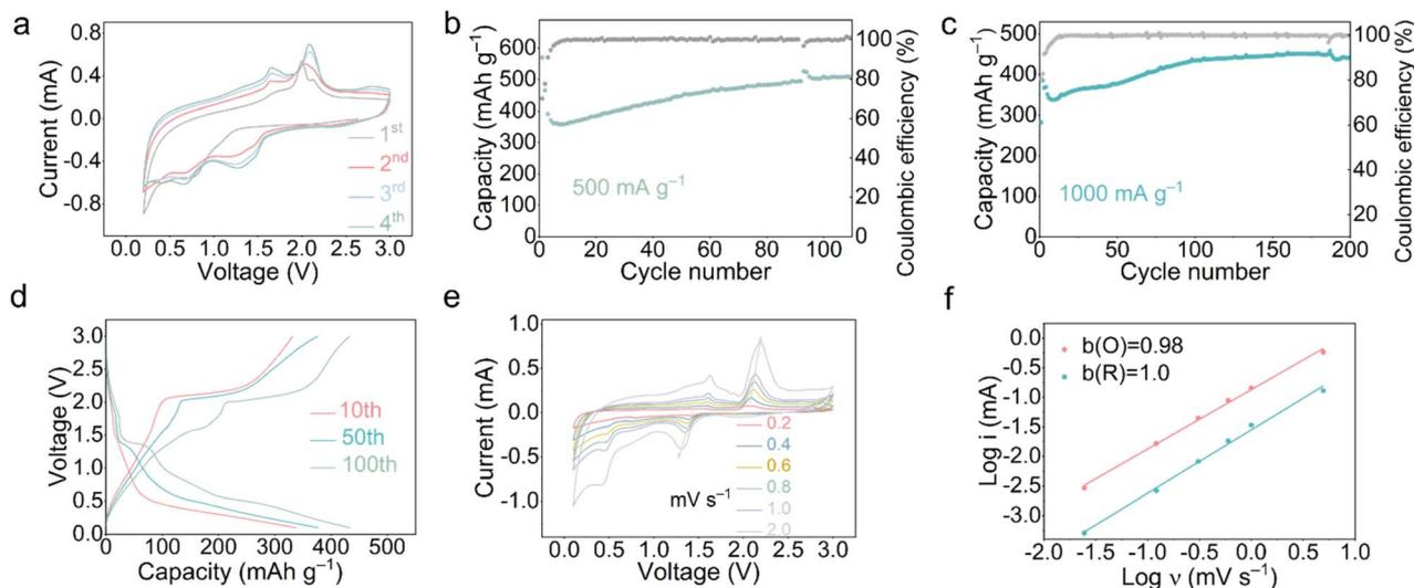
Fig. 3 Electrochemical performances of hierarchical  $\text{VS}_4$  nanosheets: (a) CV curves at  $0.5 \text{ mV s}^{-1}$ , cycling performance at current densities of (b)  $500 \text{ mA g}^{-1}$  and (c)  $1000 \text{ mA g}^{-1}$ , and (d) the corresponding charge-discharge profiles after different cycles at  $1000 \text{ mA g}^{-1}$ . (e) CV curves at varying scan rates and (f) the corresponding calculated values of  $b$ .
