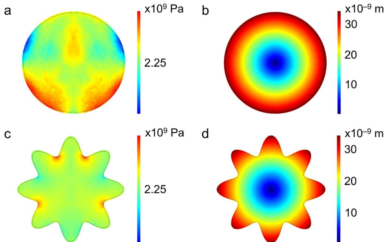
Fig. 8 FES: (a and c) stress distributions in solid spheres and hierarchical VS<sub>4</sub> nanosheets, respectively (b and d). Total displacements in solid spheres and hierarchical VS<sub>4</sub> nanosheets, respectively.
