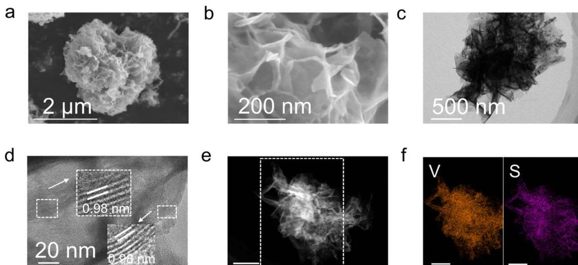
Fig. 1 Material characterization: (a and b) SEM images, (c) TEM image, (d) HRTEM image, and (e) STEM image and (f) corresponding elemental maps of V and S in hierarchical  $VS_4$  nanosheets (scale bar: (e): 500 nm, (f): 500 nm).
