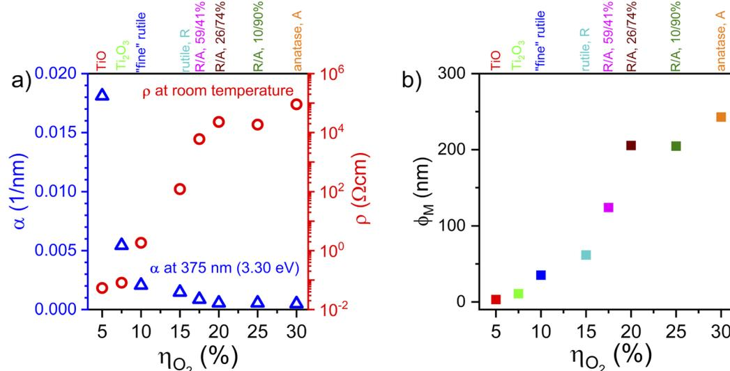
Fig. 3 Absorption coefficient (blue triangles) at  $\lambda = 375$  nm ( $h\nu = 3.30$  eV), electrical resistivity (red circles) from electrochemical impedance spectra measured at room temperature for titanium oxide thin films sputtered at different oxygen flow ratios  $\eta_{O_2}$  and oxygen partial pressures  $p_{O_2}$  (a), and figure of merit ( $\phi_M$ ) of thin films with different crystallographic structures calculated from eqn (3) (b).
