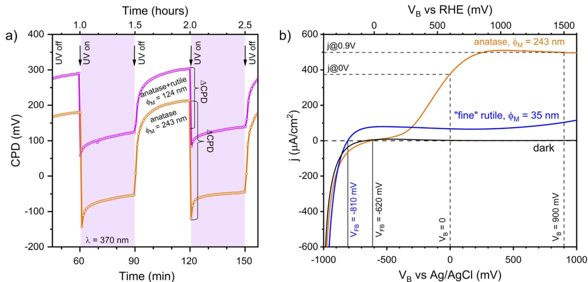
Fig. 8 Contact potential difference CPD vs. time for rutile/anatase and anatase thin films with changes under 370 nm illumination ( $\Delta$ CPD) marked (a); current density  $j$  as a function of applied bias voltage  $V_B$  in PEC (b).
