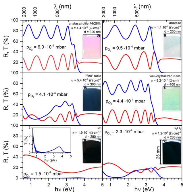
Fig. 2 Transmittance (blue) and specular reflectance (red) coefficients as a function of photon energy ( $h\nu$ ) for titanium oxide thin films obtained at different oxygen partial pressures  $p_{\text{O}_2}$ ; conductivity at room temperature ( $\sigma$ ) calculated from EIS measurements, thickness ( $d$ ) and photographs of thin films deposited on amorphous silica substrates (dimensions  $18 \times 25$  mm). In the inset: transmittance spectrum for TiO thin films.
