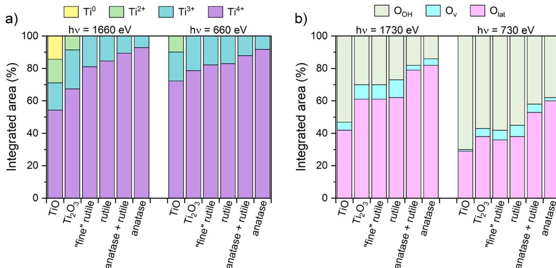
Fig. 6 Integrated areas of XPS peaks based on Gaussian fitting of Ti 2p (a) and O 1s (b) spectra presented in Fig. 5.
