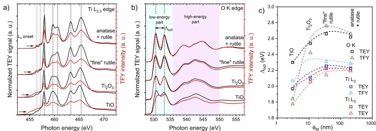
Fig. 7 Titanium L<sub>2,3</sub> (a) and oxygen K (b) edge X-ray absorption spectra after background subtraction, collected in TEY (black) and TFY (red) modes for TiO, Ti<sub>2</sub>O<sub>3</sub> and TiO<sub>2</sub> thin films with main line positions marked. Crystal field splitting  $\Delta_{\text{oct}}$  calculated as a difference in positions of  $e_g$  and  $t_{2g}$  peaks based on O K and Ti L<sub>2,3</sub> spectra in TEY and TFY modes (c) for thin films with different  $\phi_M$ .
