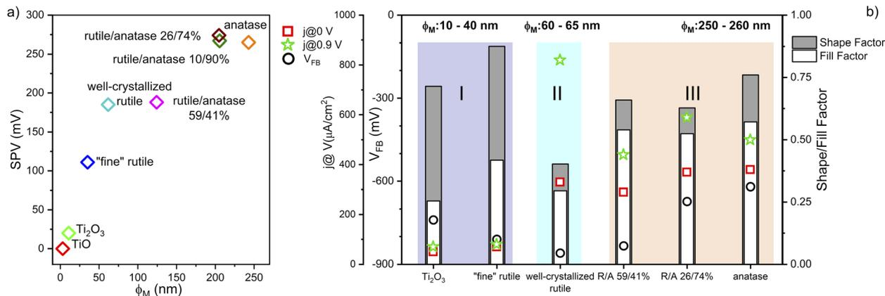
Fig. 9 Surface photovoltage SPV ( $=-\Delta\text{CPD}$ ) under 370 nm illumination as a function of figure of merit  $\phi_M$  for thin films of different phase compositions (a) and the analysis of the most important parameters of PEC performance,  $V_{\text{FB}}$  – flat band potential,  $j$  – current density upon white light illumination, shape and fill factor (b).
