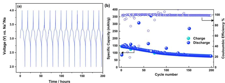
Fig. 5 (a) Voltage profile; (b) cycling performance (specific capacity and coulombic efficiency) of a Na|CPE20NAO|Na<sub>x</sub>Fe[Fe(CN)<sub>6</sub>] solid-state battery cell cycled at C/10 at 55 °C, within the voltage window of 2.0–4.0 V.
