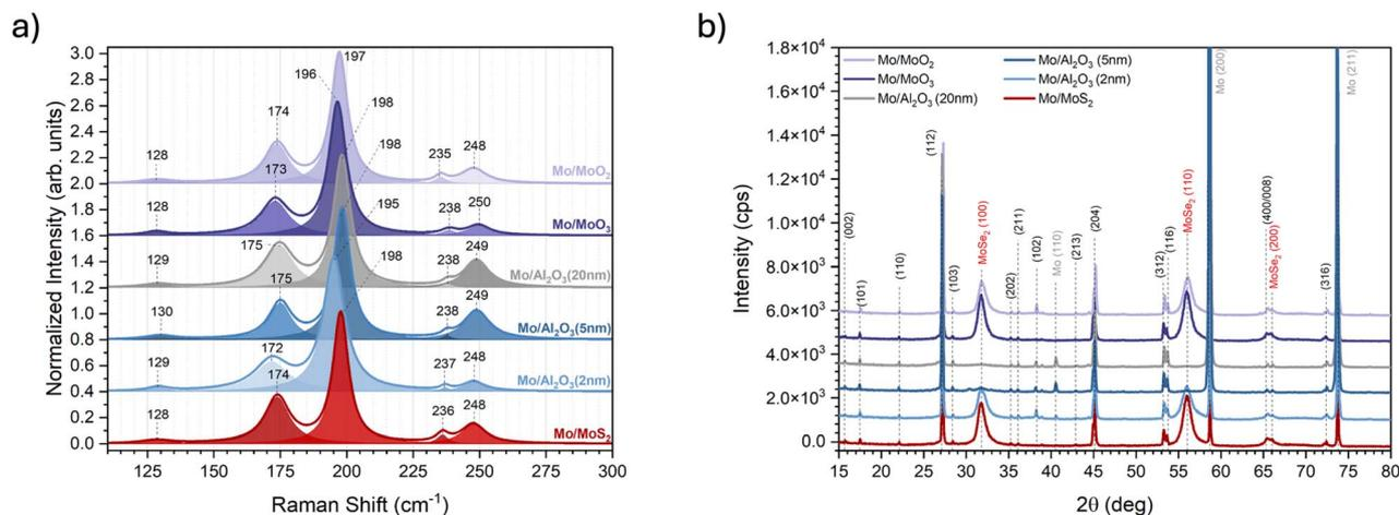
Fig. 2 (a) Deconvoluted Raman peaks and (b) crystallographic patterns of Li-ACZTSSe-based devices on flexible Mo foil with MoS<sub>2</sub> (dark red line), 2 nm Al<sub>2</sub>O<sub>3</sub> (light blue line), 5 nm Al<sub>2</sub>O<sub>3</sub> (blue line), 20 nm Al<sub>2</sub>O<sub>3</sub> (grey line), MoO<sub>3</sub> (purple line), and MoO<sub>2</sub> (lilac line) as interfacial layers.
