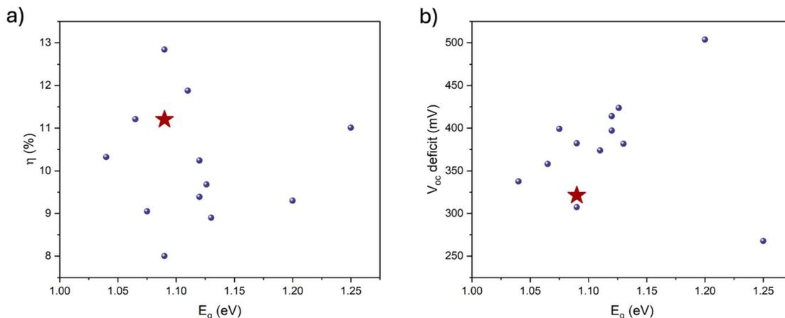
Fig. 6 (a) Record efficiencies of kesterite solar cells on flexible Mo foil and (b)  $V_{OC}$  deficit of the corresponding devices as a function of  $E_g$ .<sup>16–18,39</sup> The results of this work are highlighted with a red star.
