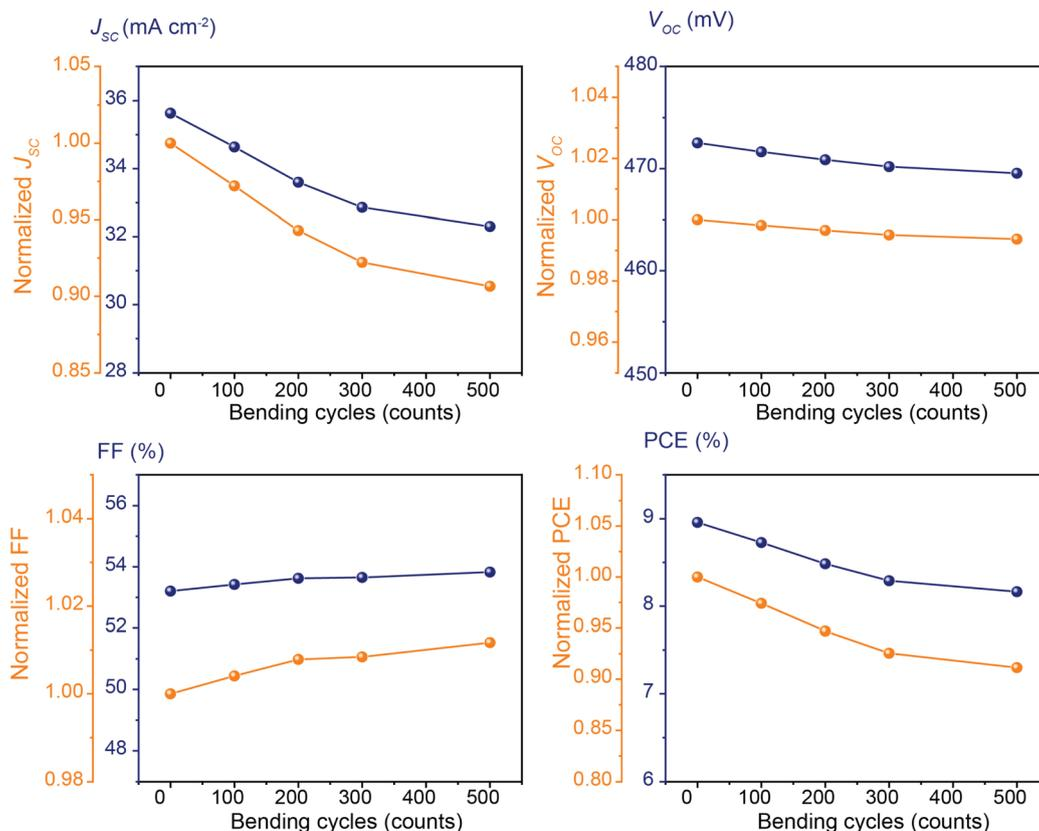
Fig. 7 Photovoltaic parameters of flexible kesterite solar cells fabricated on Mo/MoO<sub>3</sub> substrates after bending tests with varying cycle counts (bending radius fixed at 1 cm for 2.5 × 2.5 cm<sup>2</sup> devices). Changes in  $J_{sc}$ ,  $V_{oc}$ , FF, and PCE are shown, along with their normalized values.
