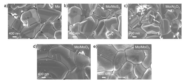
Fig. 4 Top-view SEM images of the absorbers grown on (a) Mo foil, (b) Mo foil/MoS<sub>2</sub>, (c) Mo foil/2 nm Al<sub>2</sub>O<sub>3</sub>, (d) Mo foil/MoO<sub>3</sub>, and (e) Mo foil/ MoO<sub>2</sub>.
