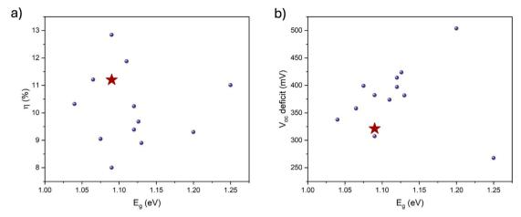
Fig. 6 (a) Record efficiencies of kesterite solar cells on flexible Mo foil and (b)  $V_{\rm OC}$  deficit of the corresponding devices as a function of  $E_{\rm g}$ . The results of this work are highlighted with a red star.
