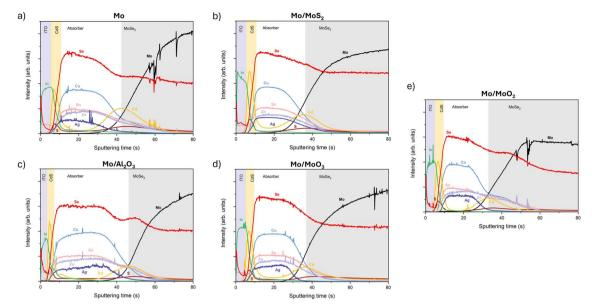
GDOES profiles of devices with (a) Mo foil, (b) Mo foil/MoS<sub>2</sub>, (c) Mo foil/2 nm  $Al_2O_3$ , (d) Mo foil/MoO<sub>3</sub>, and (e) Mo foil/MoO<sub>2</sub> as substrates.
