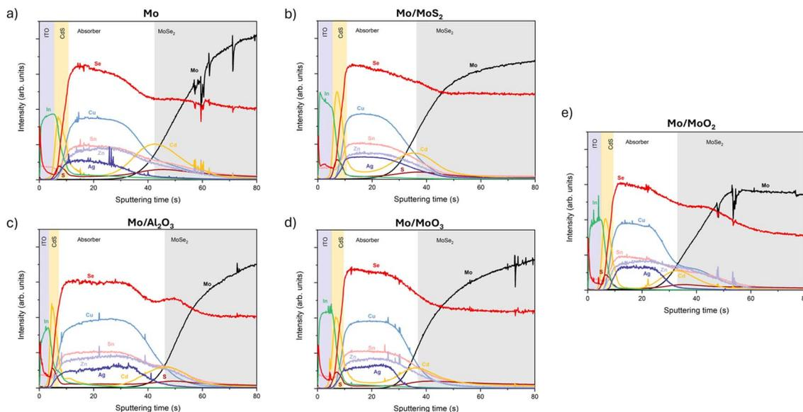
Fig. 3 GDOES profiles of devices with (a) Mo foil, (b) Mo foil/MoS<sub>2</sub>, (c) Mo foil/2 nm Al<sub>2</sub>O<sub>3</sub>, (d) Mo foil/MoO<sub>3</sub>, and (e) Mo foil/MoO<sub>2</sub> as substrates.
