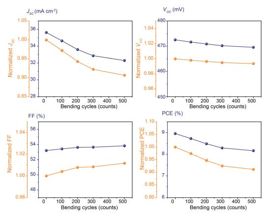
Fig. 7 Photovoltaic parameters of flexible kesterite solar cells fabricated on Mo/MoO<sub>3</sub> substrates after bending tests with varying cycle counts (bending radius fixed at 1 cm for  $2.5 \times 2.5$  cm<sup>2</sup> devices). Changes in  $J_{SC}$ ,  $V_{OC}$ , FF, and PCE are shown, along with their normalized values.
