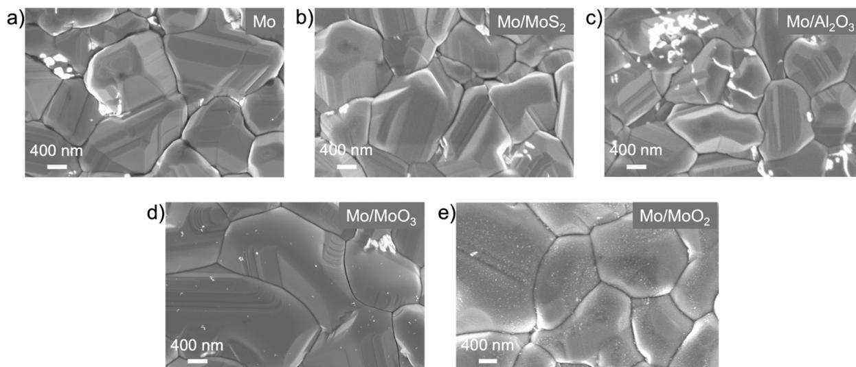
Fig. 4 Top-view SEM images of the absorbers grown on (a) Mo foil, (b) Mo foil/MoS<sub>2</sub>, (c) Mo foil/2 nm Al<sub>2</sub>O<sub>3</sub>, (d) Mo foil/MoO<sub>3</sub>, and (e) Mo foil/MoO<sub>2</sub>.
