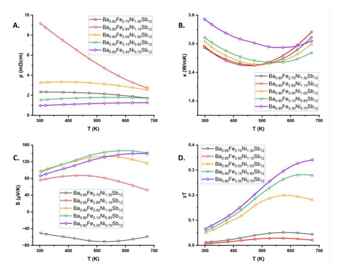
Fig. 8 Thermoelectric properties of the Ba<sub>0.9</sub>Fe<sub>3±x</sub>Ni<sub>1±x</sub>Sb<sub>12</sub> skutterudites. (A) Electrical resistivities in milliohm-centimeters. (B) Thermal conductivities in watts per meter kelvin. (C) Seebeck coefficients in microvolts per kelvin. (D) Unitless figures of merit zT.
