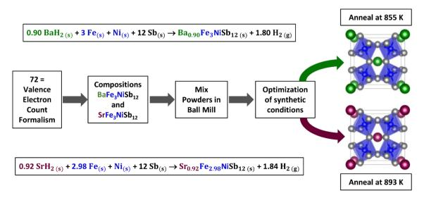
Fig. 1 Overview of the preparation of skutterudites as performed herein. Samples were heated to their annealing temperature within 6 hours and annealed for 16 hours.
