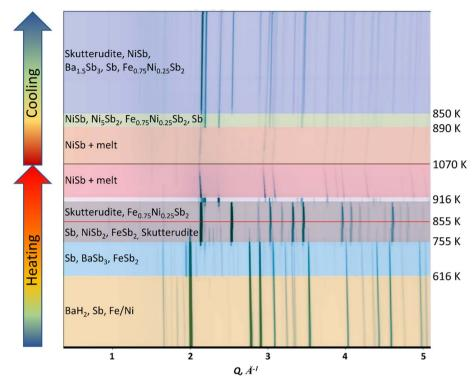
Fig. 2 High-temperature in situ powder X-ray diffraction data obtained upon heating to 1070 K and subsequent cooling of a BaH<sub>2</sub>, Sb, Fe, Ni precursors mixture. Data represented as a contour plot, and each horizontal section corresponds to a PXRD pattern where darker shading indicates higher relative diffraction intensity. The temperature ranges with distinct crystalline phases present are highlighted in yellow, light blue, grey, pink, orange, light green, and blue.
