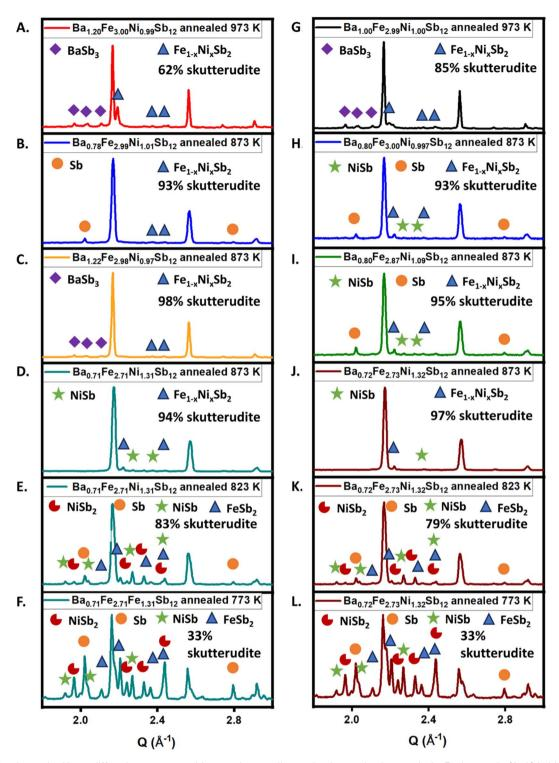
Fig. 4 Abridged powder X-ray diffraction patterns with non-skutterudite peaks denoted using symbols. Each sample (A–L) is identified by its reaction stoichiometry and annealing temperature. The wt% of skutterudite phase was estimated using full-profile fitting. This is the experimental data used to validate the response surface modeling functionality of JMP Pro 16 for the optimization of synthetic conditions to form  $BaFe_3NiSb_{12}$ .
