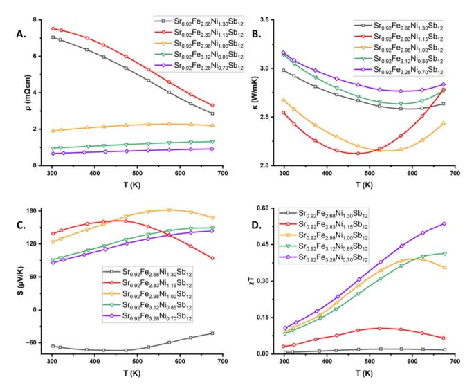
Fig. 9 Thermoelectric Properties of Sr<sub>0.92</sub>Fe<sub>2.98±x</sub>Ni<sub>1±x</sub>Sb<sub>12</sub> skutterudites. (A) Electrical resistivities in milliohm-centimeters. (B) Thermal conductivities in watts per meter kelvin. (C) Seebeck coefficients in microvolts per kelvin. (D) Unitless figures of merit, zT.
