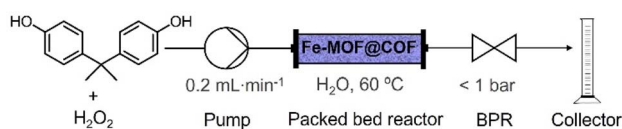
Scheme 1 Continuous Fenton reaction and capture of BPA.
