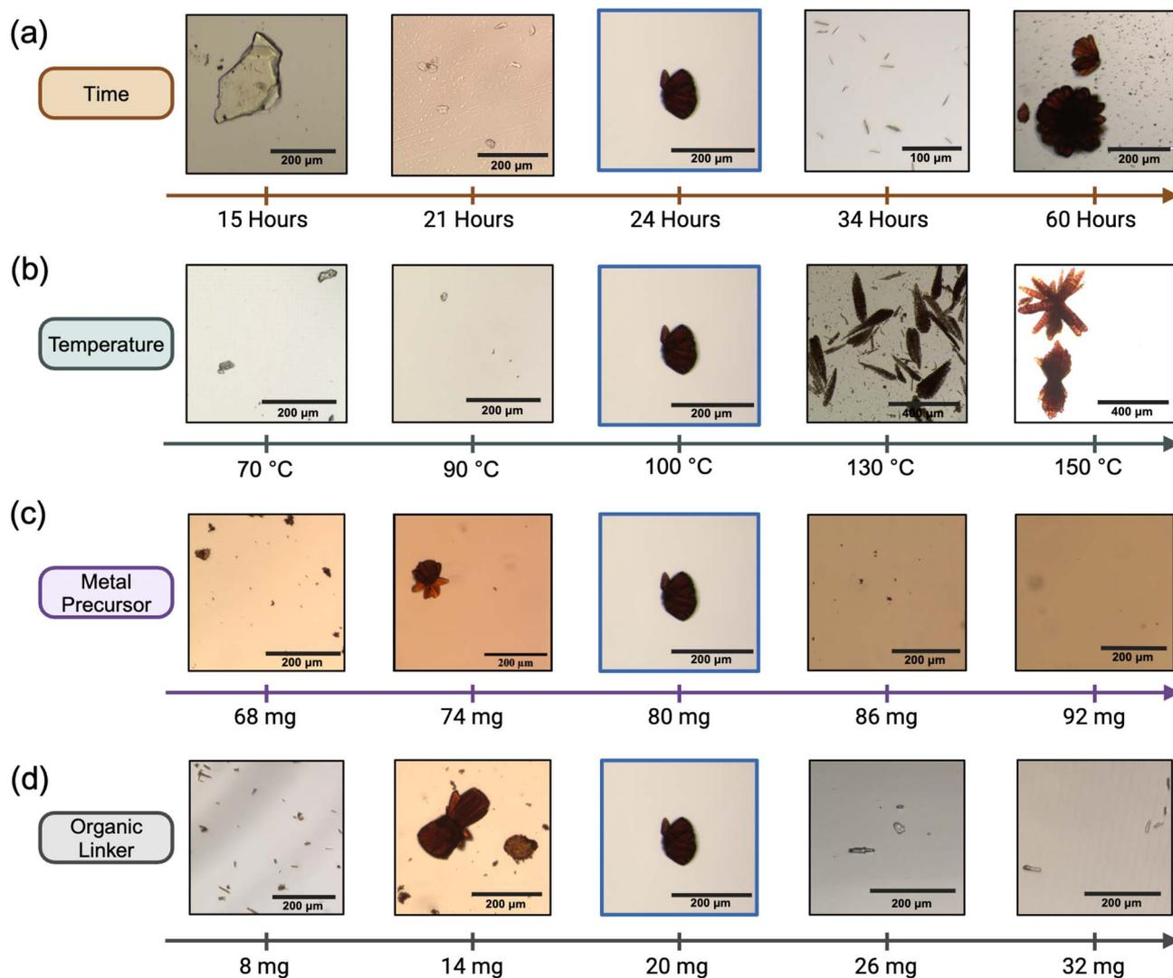
Fig. 3 (a–d) Variation in shape and shape and morphology of the synthesized crystals and different synthesis conditions: (a) time, (b) temperature, (c) metal precursor, and (d) organic linker while keeping the other parameters constant.
