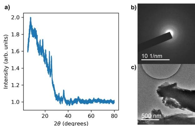
Fig. 3 (a) XRD pattern, (b) TEM diffraction pattern and (c) high resolution TEM image of solution-based LiPON.
