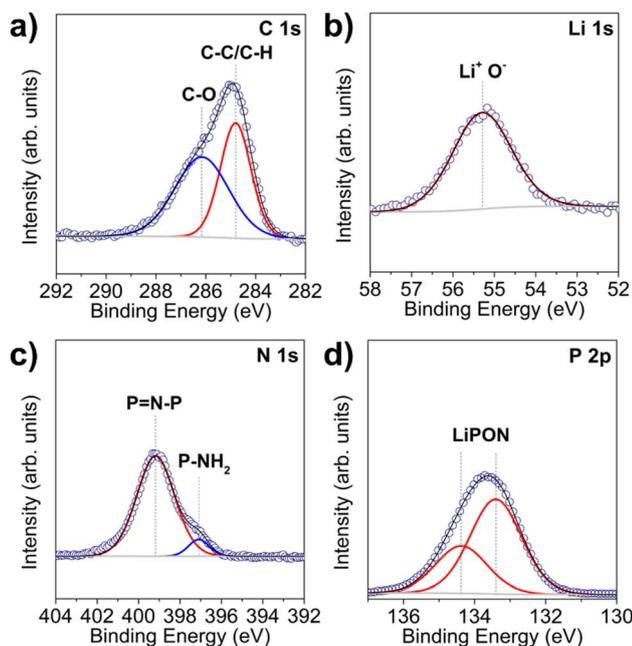
Fig. 4 High-resolution XPS (a) C 1s, (b) Li 1s, (c) 1s, and (d) P 2p spectra of solution-made LiPON after 7 minutes of Ar<sup>+</sup> sputtering.
