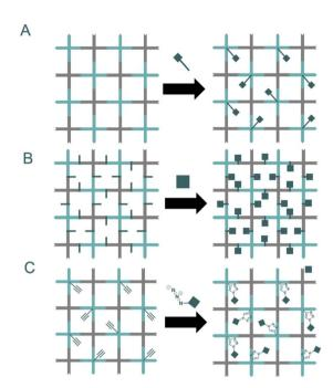
Fig. 10 Post synthetic modification of COFs: incorporation of side chains *via* isosteric substitution of the core (A) or incorporation of pendant moieties (B). Finally, click chemistry approaches allow the rapid, quantitative functionalization of COFs (C).
