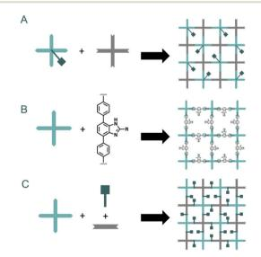
Fig. 9 Different strategies for *de novo* construction of COFs: incorporation of a functionalizable moiety in a well-known core (A), incorporation of 4,7-disubstituted benzimidazole as building block core (B), assembly of the network using a multicomponent reaction (C).
