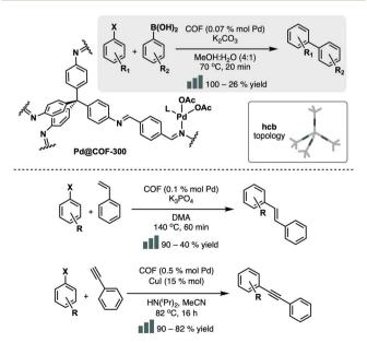
Fig. 11 Material and catalytic reaction studied in ref. 60.
