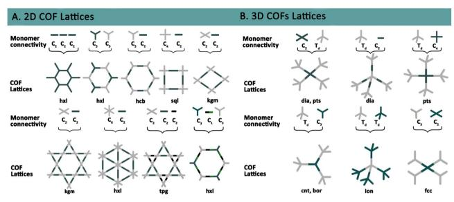
Fig. 3 Topological diagrams illustrating representative designs of 2D and 3D COFs.
