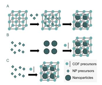
**Fig. 16** Different strategies for encapsulation of nanoparticles inside COFs. Ship-in-bottle approach (A), ship-around-bottle approach (B) and one-step synthesis approach (C).
