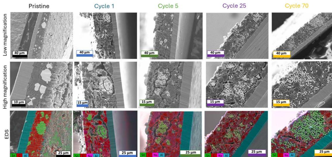
Fig. 4 Ion-beam milled SEM cross-sections with corresponding EDS for pristine SnHC64 electrodes and cycled electrodes (1<sup>st</sup>, 5<sup>th</sup>, 25<sup>th</sup> and 70<sup>th</sup> cycle in the de-sodiated state).
