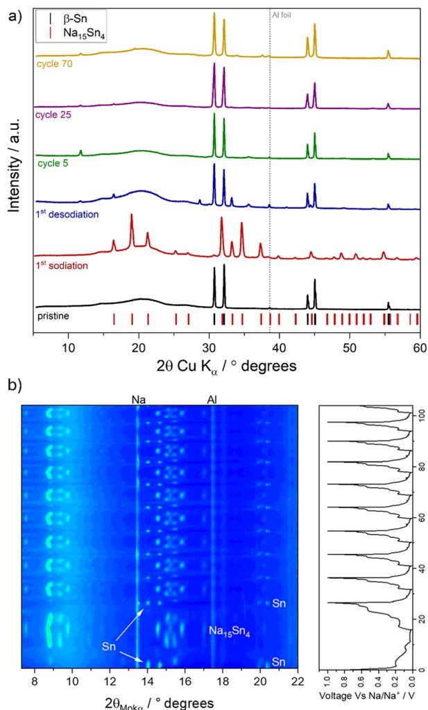
Fig. 6 (a) *Ex situ* XRD patterns of SnHC82 electrodes in the pristine and cycled states. (b) *Operando* XRD over ten cycles of the SnHC82 electrode cycled at 50 mA g<sup>-1</sup> (1<sup>st</sup> cycle) and at 100 mA g<sup>-1</sup> (10<sup>th</sup> cycle) in Na half-cell using 1 M NaPF<sub>6</sub> in diglyme as electrolyte.
