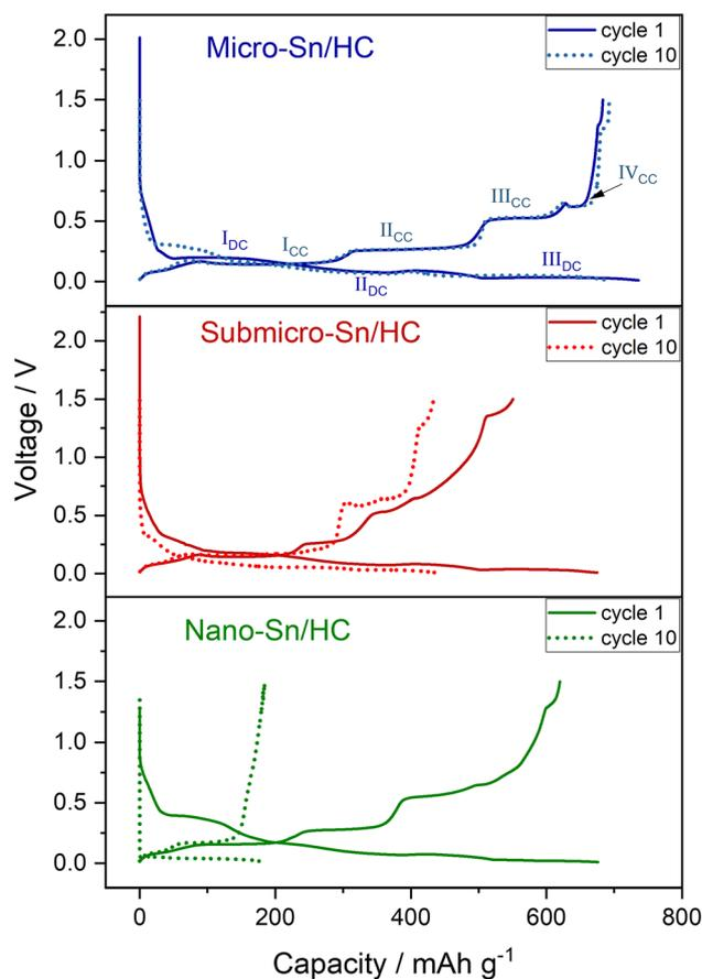
Fig. 2 Galvanostatic cycling of micro-, submicro- and nano-Sn/HC electrodes (8 : 2 wt%) cycled at  $50 \text{ mA g}^{-1}$  ( $1^{\text{st}}$  cycle) and at  $100 \text{ mA g}^{-1}$  ( $10^{\text{th}}$  cycle). Tests conducted at  $25^\circ\text{C}$  within the  $0.01\text{--}1.5$  V range. Electrolyte:  $1 \text{ M NaPF}_6$  in diglyme.
