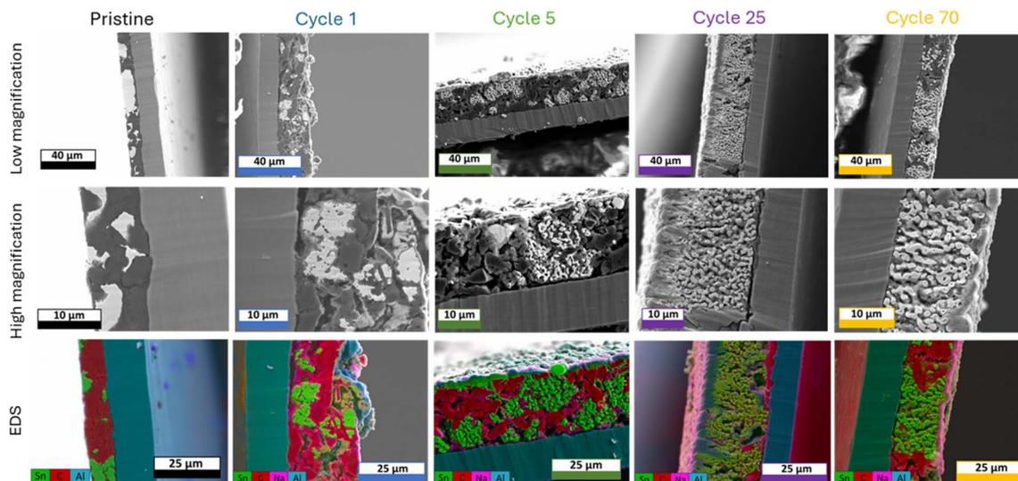
Fig. 3 Ion-beam milled SEM cross-sections with corresponding EDS for pristine SnHC82 electrodes and cycled electrodes (1<sup>st</sup>, 5<sup>th</sup>, 25<sup>th</sup> and 70<sup>th</sup> cycle in the de-sodiated state).
