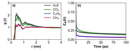
Fig. 12 (a) RDF between gas molecules and N atoms in PPN and (b) residence autocorrelation functions  $C_{\rm P}(t)$  for gas molecules within cutoff distances of  $\sim$ 1.0 nm from N atoms in the polymer blends. The simulation results were obtained for pure gases in PTMSP-20PPN blends at 298 K, with data averaged over five independent samples.
