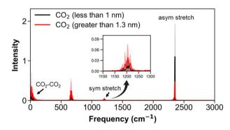
Fig. 13 Power spectra for CO<sub>2</sub> molecules within the polymer matrix: (a) within a 1 nm cutoff distance from N atoms and (b) beyond 1.3 nm from N atoms. These cutoff distances were determined based on RDF calculations, as shown in Fig. 12. The spectra were derived from molecular dynamics simulations of CO2 in PTMSP-20PPN blends at 298 K and 1 bar and averaged over five samples. Shaded regions represent standard deviation.
