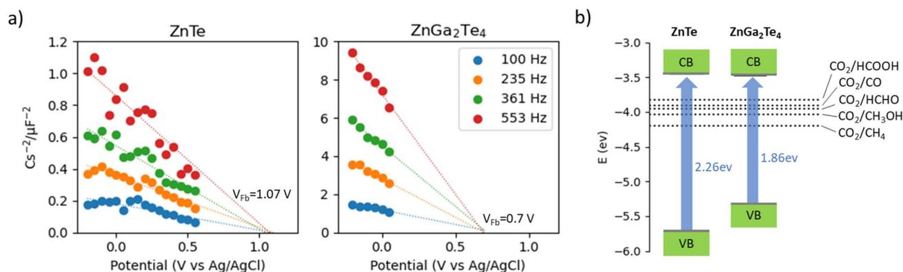
Fig. 8 Mott-Schottky analysis (a) energy band position characterization for ZnTe and  $\text{ZnGa}_2\text{Te}_4$ . Measurements are carried out in  $\text{CO}_2$ -bubbled 0.1 M  $\text{KHCO}_3$  (pH = 6.8) and at multiple frequencies to validate the measured flat band potentials. (b) Band potentials and bandgap energy for ZnTe and  $\text{ZnGa}_2\text{Te}_4$ .
