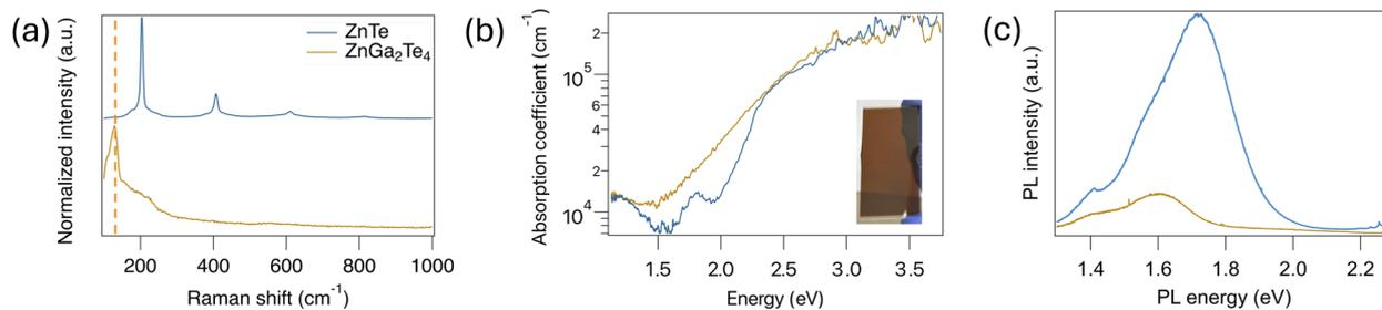
Fig. 6 Optical characterization (a) Raman scattering – dashed line indicates the A1 vibrational mode for tetragonal  $\text{ZnGa}_2\text{Te}_4$  (b) absorption coefficients ( $\alpha(E)$ ) spectra (inset is a photograph of uniform  $\text{ZnGa}_2\text{Te}_4$  thin film on FTO substrate) (c) room-temperature PL spectra.
