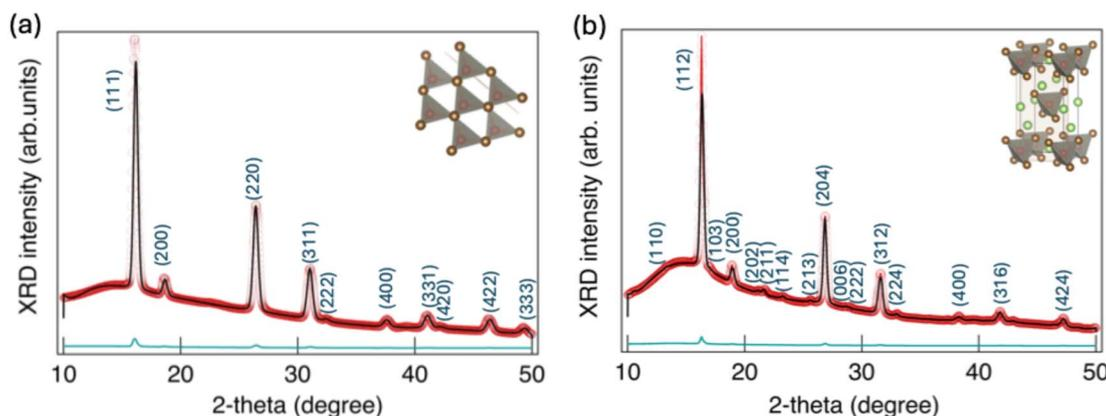
Fig. 3 Wide-angle X-ray analysis integrated wide-angle X-ray scattering pattern along with a LeBail fit to the (a) cubic  $\text{Ga:ZnTe}$  and (b) tetragonal  $\text{ZnGa}_2\text{Te}_4$  structure (here, black, red and cyan color represent calculated, experimental and difference spectrum of the refinement spectra) ( $\lambda = 0.97625$  Å).
