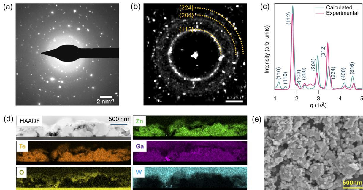
Fig. 4 Electron microstructure (a) TEM SAED pattern, (b) 4D-STEM virtual SAED (Bragg vector map) from the  $\text{ZnGa}_2\text{Te}_4$  film, (c) experimental 1D diffraction pattern azimuthally integrated from 4D-STEM along with the simulated diffraction pattern, (d) STEM HAADF image and corresponding EDS elemental maps and (e) SEM top view of  $\text{ZnGa}_2\text{Te}_4$  thin films.
