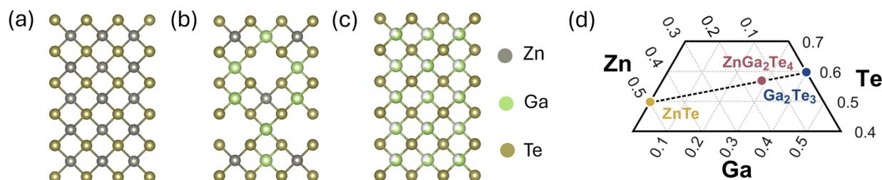
Fig. 1 Crystal structure (a) zinc blende derived ZnTe (b) tetragonal ZnGa<sub>2</sub>Te<sub>4</sub> (c) defective Ga<sub>2</sub>Te<sub>3</sub> (d) chemical formulas and ternary phase diagram showing the compositional tie-line between zincblende-derived Zn–Ga–Te materials (ZnTe)<sub>x</sub>(Ga<sub>2</sub>Te<sub>3</sub>)<sub>1-x</sub> thin film growth.
