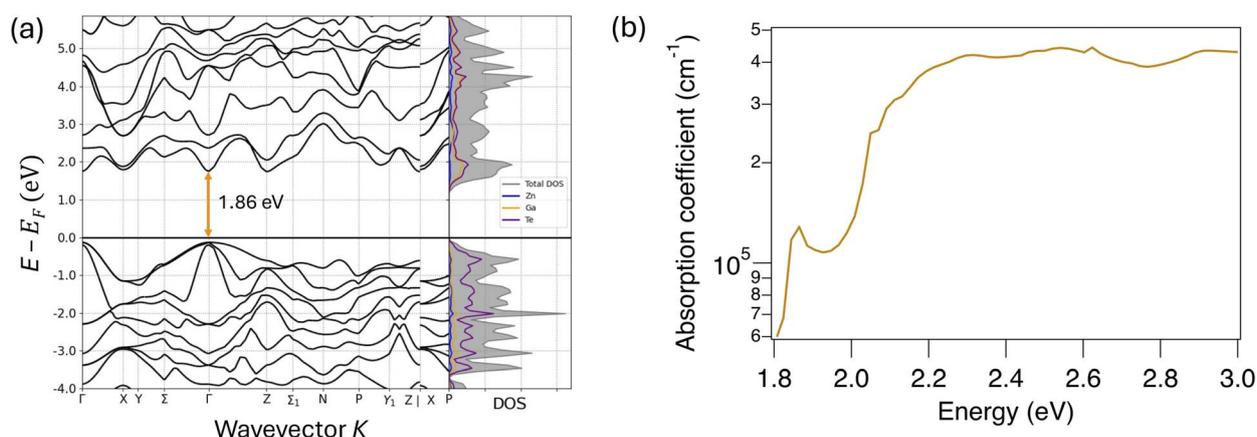
Fig. 5 DFT calculation (a) electronic band structure of  $\text{ZnGa}_2\text{Te}_4$  with total and element-resolved density of states (b) theoretically calculated absorption coefficient ( $\alpha$ ) for  $\text{ZnGa}_2\text{Te}_4$ .
