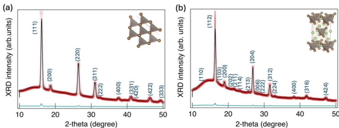
Fig. 3 Wide-angle X-ray analysis integrated wide-angle X-ray scattering pattern along with a LeBail fit to the (a) cubic Ga:ZnTe and (b) tetragonal  $\text{ZnGa}_2\text{Te}_4$  structure (here, black, red and cyan color represent calculated, experimental and difference spectrum of the refinement spectra) ( $\lambda = 0.97625$  Å).
