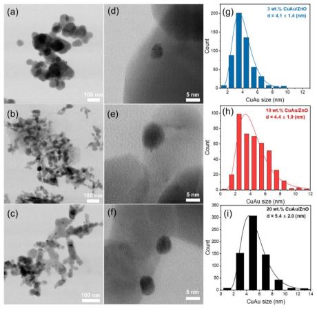
Fig. 1 Representative STEM micrographs of different loadings of the  $Cu_xAu_y$  alloy (3, 10, and 20 wt%) on a ZnO support. Overview images (a–c) and high-resolution images of  $Cu_xAu_y$  alloy nanoparticles (d–f), and corresponding particle size distributions (g–i).
