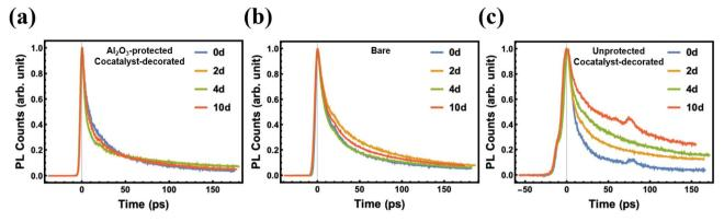
Fig. 5 TRPL signals (440-460 nm) of three sets of InGaN/GaN nanowire samples for 0, 2, 4, and 10 reaction days: (a) Al<sub>2</sub>O<sub>3</sub>-capped cocatalystdecorated nanowire samples. (b) Bare InGaN/GaN nanowire samples with no protection and decoration. (c) Unprotected cocatalyst-decorated nanowire samples
