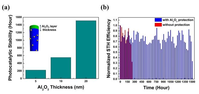
Fig. 2 (a) Photocatalytic stability of the  $Al_2O_3$ -capped cocatalyst-loaded p-InGaN nanowire samples with different  $Al_2O_3$  capping thicknesses. (b) Stability test of the cocatalyst-decorated p-InGaN nanowires with and without  $Al_2O_3$ -capping under concentrated light of 1000 mW cm<sup>-2</sup> at 70 °C temperature.
