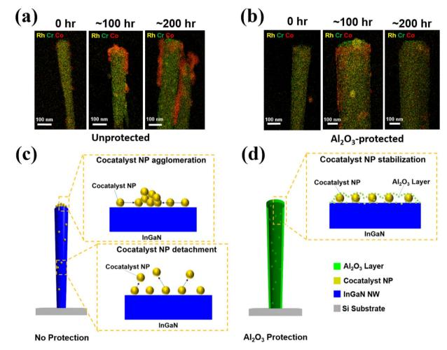
Fig. 3 EDX elemental mappings of the cocatalyst-loaded samples for different reaction durations (a) without and (b) with  $Al_2O_3$  protection. The cocatalyst NPs are agglomerated in the case of no  $Al_2O_3$  protection. Schematic depictions of the (c) cocatalyst NP displacement in the unprotected nanostructure and (d) cocatalyst stabilization effect by the  $Al_2O_3$  protection layer.
