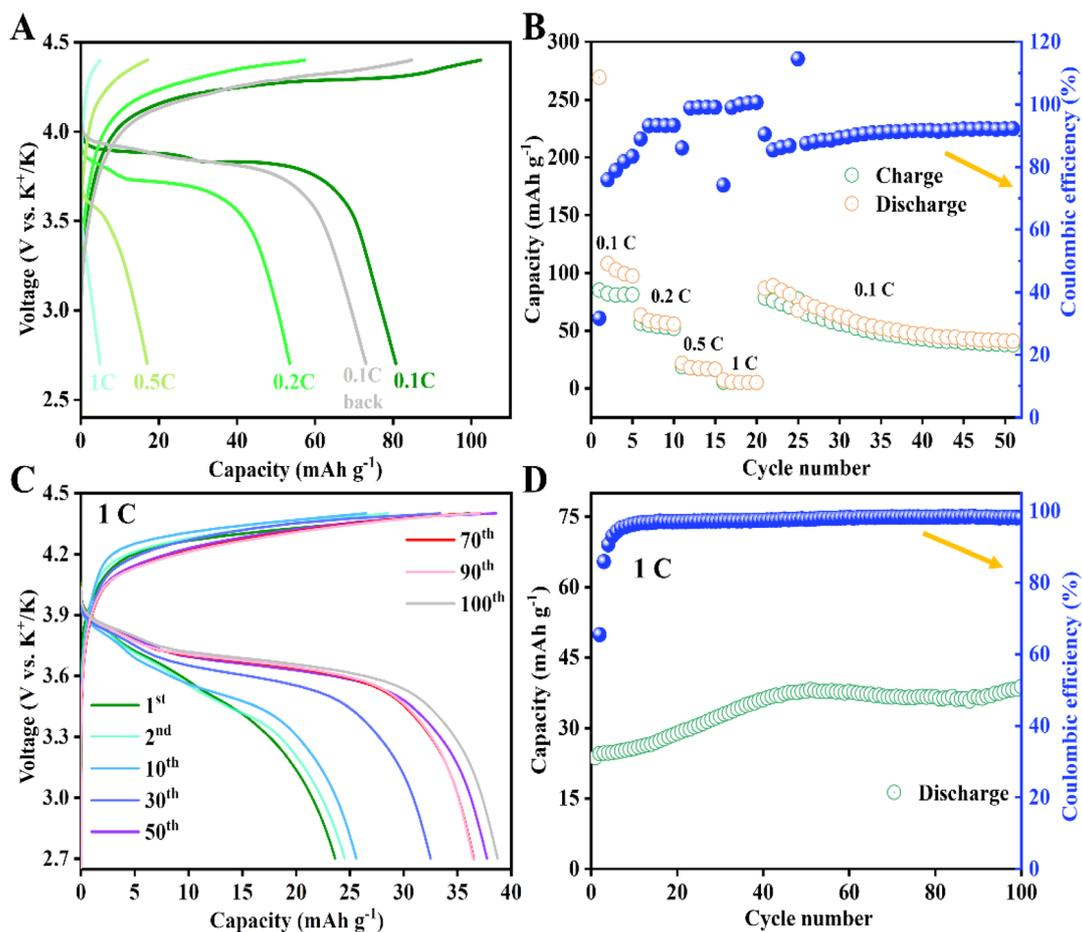
Fig. 4 Electrochemical performance of K||FSI:FSI||PW cells between the operation voltage of 4.4–2.7 V vs. K<sup>+</sup>/K at 20 °C ± 2 °C. (A) Charge and discharge curves, and (B) rate capability from 0.1C to 1C and corresponding CE, (C) 1<sup>st</sup>, 2<sup>nd</sup>, and from 10<sup>th</sup> to 100<sup>th</sup> charge–discharge curves, and (D) cycling performance and corresponding CE at 1C.
