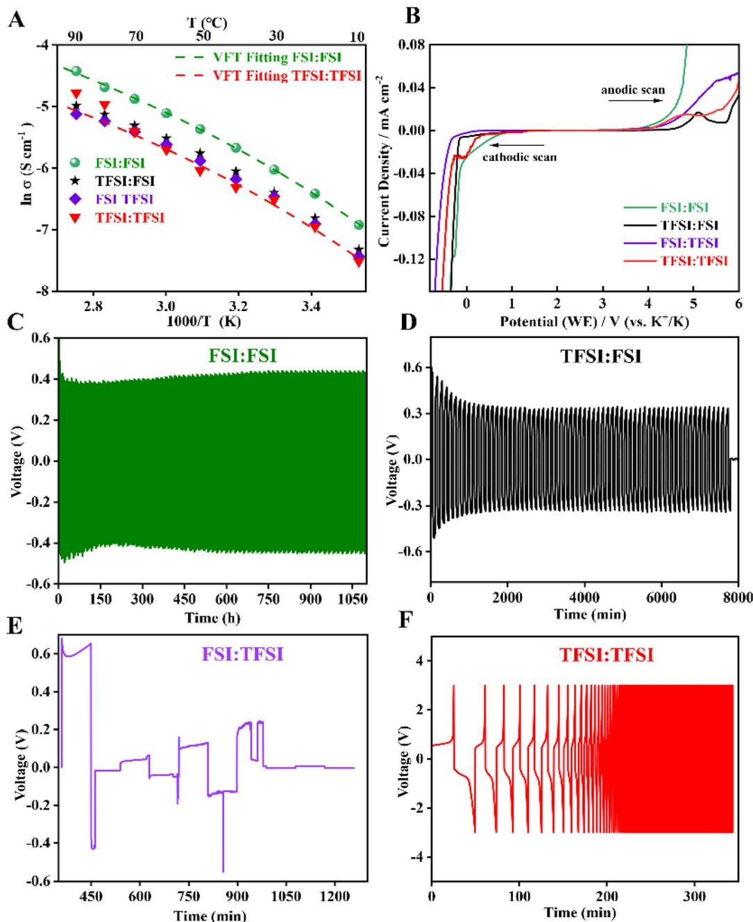
Fig. 2 (A) Temperature-dependent ionic conductivity, and (B) anodic and cathodic LSV curves (Al foil as working electrode, K as counter and reference electrode, scan rate of  $0.1 \text{ mV s}^{-1}$ ). Stripping/plating cycles in symmetrical K||solvent-free SPE||K cells at  $20^\circ \text{C}$  and current densities of  $0.1 \text{ mA cm}^{-2}$ : (C) FSI:FSI, (D) TFSI:FSI, (E) TFSI:FSI, (F) TFSI:FSI. Note the different scales on the x and y axes.
