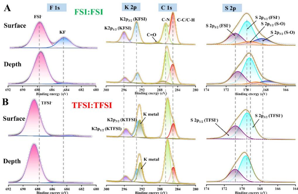
Fig. 6 XPS of the K metal surface and bulk (depth of 8 nm, Ar<sup>+</sup> etching speed of 0.8 nm min<sup>-1</sup>) after immersing for 28 days in (A) KFSI:Pyr<sub>120</sub>FSI or (B) KTFSI:Pyr<sub>120</sub>TFSI solutions (the grey open points represent the experimental data, and the solid lines represent the fitting results).
