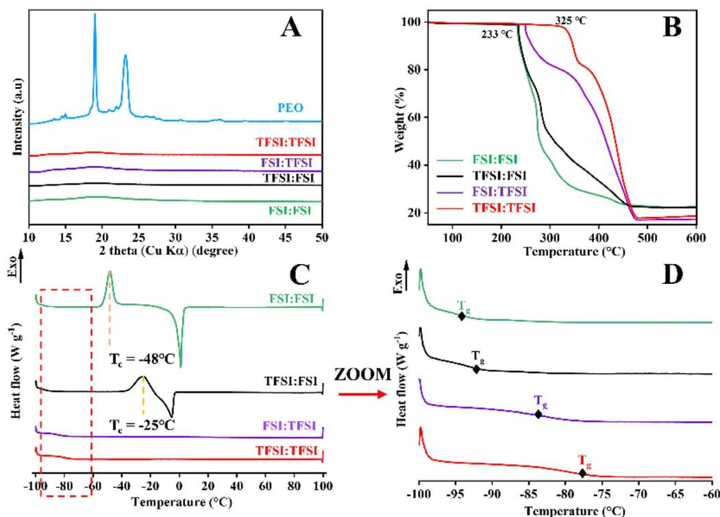
Fig. 1 (A) XRD patterns of all solvent-free SPEs and pure PEO, (B) TGA curves (heating rate of 5 K min<sup>-1</sup>, inert N<sub>2</sub> atmosphere), (C) DSC curves (heating cycles between -100 °C and 100 °C, heating rate of 5 K min<sup>-1</sup>, for all solvent-free SPEs), and (D) enlarged image of the selected area in (C).
