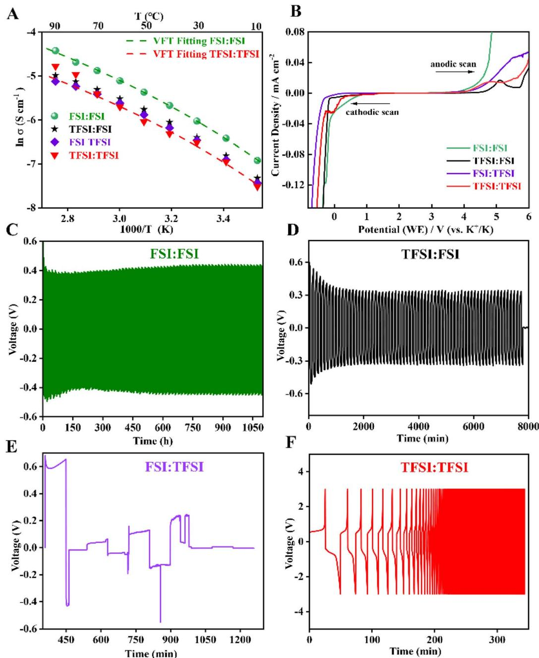
Fig. 2 (A) Temperature-dependent ionic conductivity, and (B) anodic and cathodic LSV curves (Al foil as working electrode, K as counter and reference electrode, scan rate of  $0.1 \text{ mV s}^{-1}$ ). Stripping/plating cycles in symmetrical K||solvent-free SPE||K cells at  $20 \text{ }^\circ\text{C}$  and current densities of  $0.1 \text{ mA cm}^{-2}$ : (C) FSI:FSI, (D) FSI:TFSI, (E) TFSI:FSI, (F) TFSI:FSI. Note the different scales on the x and y axes.
