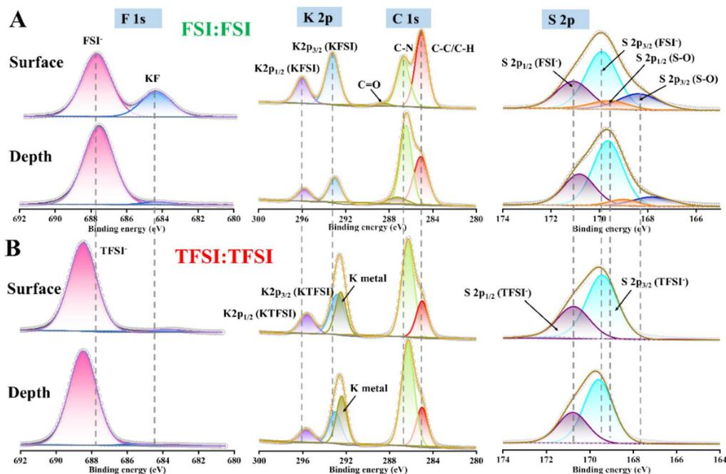
Fig. 6 XPS of the K metal surface and bulk (depth of 8 nm, Ar<sup>+</sup> etching speed of 0.8 nm min<sup>-1</sup>) after immersing for 28 days in (A) KFSI:Pyr<sub>12</sub>O<sub>1</sub>FSI or (B) KTFSI:Pyr<sub>12</sub>O<sub>1</sub>TFSI solutions (the grey open points represent the experimental data, and the solid lines represent the fitting results).
