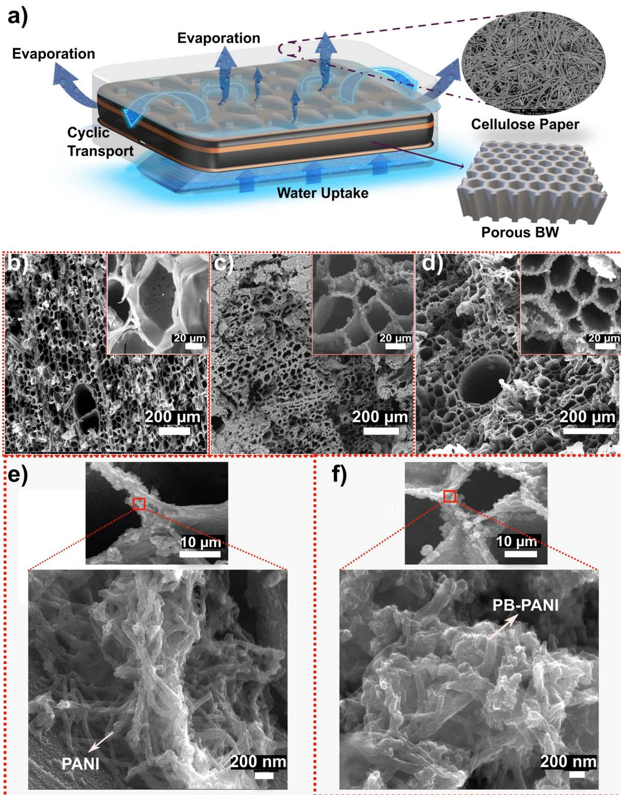
**Fig. 1** (a) Schematic illustration of the CTHG device demonstrating water absorption, transportation, and evaporation, with inset highlighting the cellulose paper and balsa wood (BW) framework as the principal energy harvesting element. (b) SEM image of D-BW; (c) SEM image of PANI-BW; (d) SEM image of PB-PANI-BW. High-magnification SEM images depicting (e) PANI and (f) PB-PANI nanostructures on the BW surface.
