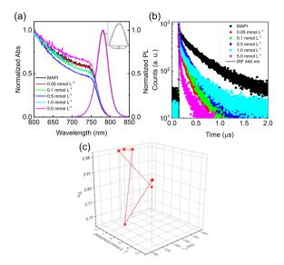
Fig. 5 (a) Electronic absorption and steady-state PL spectra, (b) TrPL decays ( $\lambda_{\rm exc}=445$  nm and  $\lambda_{\rm PL}=780$  nm), and (c) obtained charge-carrier lifetimes and disorder parameters as a function of the salophen concentration for MAPbl<sub>3</sub> and MAPbl<sub>3</sub>: salophen (0.05 to 5.0 mmol L<sup>-1</sup>) films.
