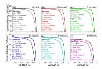
Fig. 6 J-V curves in forward and backward scan directions under illumination (100 mW cm<sup>-2</sup>) (solid lines) and in the dark (dashed lines) of the best-performing PSCs for each salophen concentration used as an antisolvent: (a) control, (b) 0.05 mmol L<sup>-1</sup>, (c) 0.1 mmol L<sup>-1</sup>, (d) 0.5 mmol L<sup>-1</sup>, (e) 1.0 mmol L<sup>-1</sup>, and (f) 5.0 mmol L<sup>-1</sup>.
