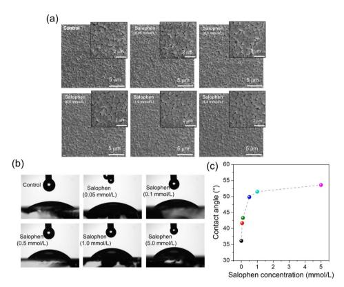
Fig. 4 (a) FEG-SEM images of FTO|c-TiO<sub>2</sub>|meso-TiO<sub>2</sub>|MAPbl<sub>3</sub> (control) and FTO|c-TiO<sub>2</sub>|meso-TiO<sub>2</sub>|MAPbl<sub>3</sub> : salophen (from 0.05 to 5.0 mmol  $L^{-1}$ ) samples. Scale bars indicate 5  $\mu$ m in FEG-SEM images. FEG-SEM images are also shown in the insets, with scale bars representing 2  $\mu$ m. (b) Contact angle images and (c) contact angle as a function of salophen concentration.
