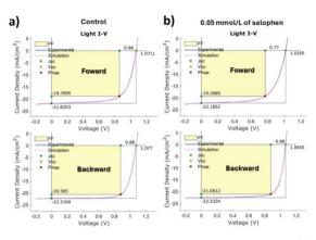
Fig. 8 J-V data and simulation of best-performing PSCs for MAPbI<sub>3</sub> (control; (a)) and MAPbI<sub>3</sub>:salophen (0.05 mmol L<sup>-1</sup>; (b)) in backward and forward scans, according to the solar cell equivalent circuit. The yellow square represents the maximum power, related to the FF.
