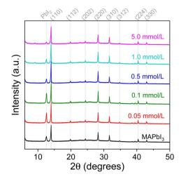
Fig. 3 XRD patterns of the pristine MAPbl<sub>3</sub> (control) and MAPbl<sub>3</sub>: salophen  $(0.05 \text{ to } 5.0 \text{ mmol L}^{-1})$  films.
