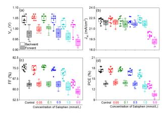
Fig. 7 Statistical distributions of (a) open circuit voltage  $(V_{oc})$ , (b) shortcircuit current density  $(J_{sc})$ , (c) fill factor (FF), and (d) PCE obtained from nine devices for each concentration of salophen (from 0.05 to 5.0 mmol L<sup>-1</sup>) used as antisolvent for backward and forward scans.
