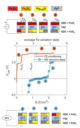
Fig. 5 Electrochemical characterisation of a symmetrical cell with two GDC +  $FeO_x$  electrodes at 650 °C un UHV. The orange line shows the conditioning step, and the blue symbols represent the cell OCV after subsequent galvanostatic steps with the negative current. The sketches represent the different phase equilibria at the top and bottom electrodes during CE conditioning (top) and stepwise reduction of the upper electrode (bottom).
