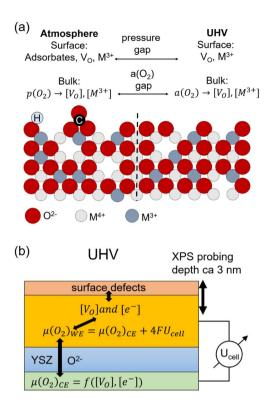
Fig. 1 (a) Simplified sketch of surface and bulk defects at an oxygen  $MO_{2-\delta}$  surface sample in (left) atmosphere and (right) vacuum. (b) Schematic of the coupling of the oxygen chemical potentials and point defects in a solid oxide cell in UHV.
