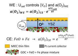
Fig. 3 Sketched principle of the working electrode oxygen activity control in the EXACT model cell in UHV.
