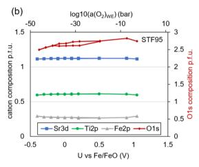
Fig. 11 Surface cation composition as function of cell bias at 400 °C determined by XPS for (a) STF100 and (b) STF95.
