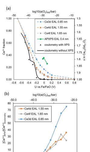
Fig. 9 (a)  $Ce^{3+}$  fraction (left y axis) and oxygen stoichiometry (right y axis) of the GDC10 film, determined by XPS (symbols) and bulk coulometry (black line) as function of cell voltage (lower x-axis) at 510 °C. The corresponding  $a(O_2)_{WF}$  values are given in the upper x-axis. The green data series was taken from synchrotron-based ambient-pressure XPS measurements in literature.11 (b) Ratio of surface and bulk Ce3+ fraction.
