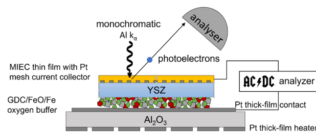
Fig. 4 Sketch of the combined electrochemical and XPS investigations of the EXACT model cell.
