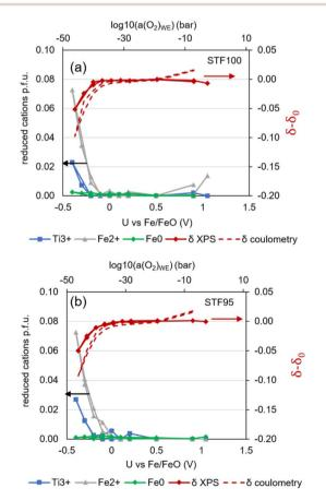
Fig. 13 Concentrations of reduced cations (left y-axis, normalised as in Fig. 11 to Sr + Ti + Fe = 100% and change in oxygen stoichiometry (right y-axis) for (a) STF100 and (b) STF95.
