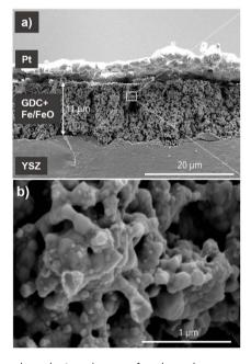
Fig. 6 Secondary electron image of a cleaved cross section of the symmetric porous electrode after electrochemical characterization in UHV (reduced after measurement). (a) 8k magnification (b) 116k magnification.
