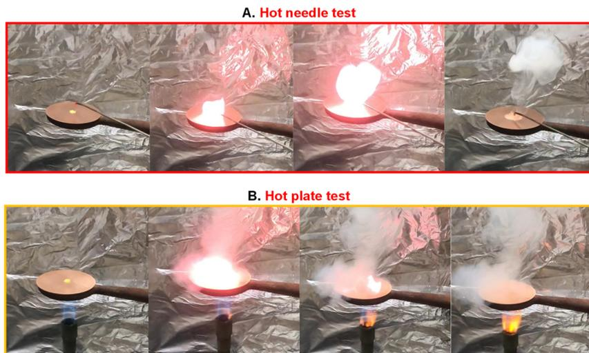
Fig. 5 (A) Hot needle test for K<sub>2</sub>DNMNAT. (B) Hot plate test for K<sub>2</sub>DNMNAT.
