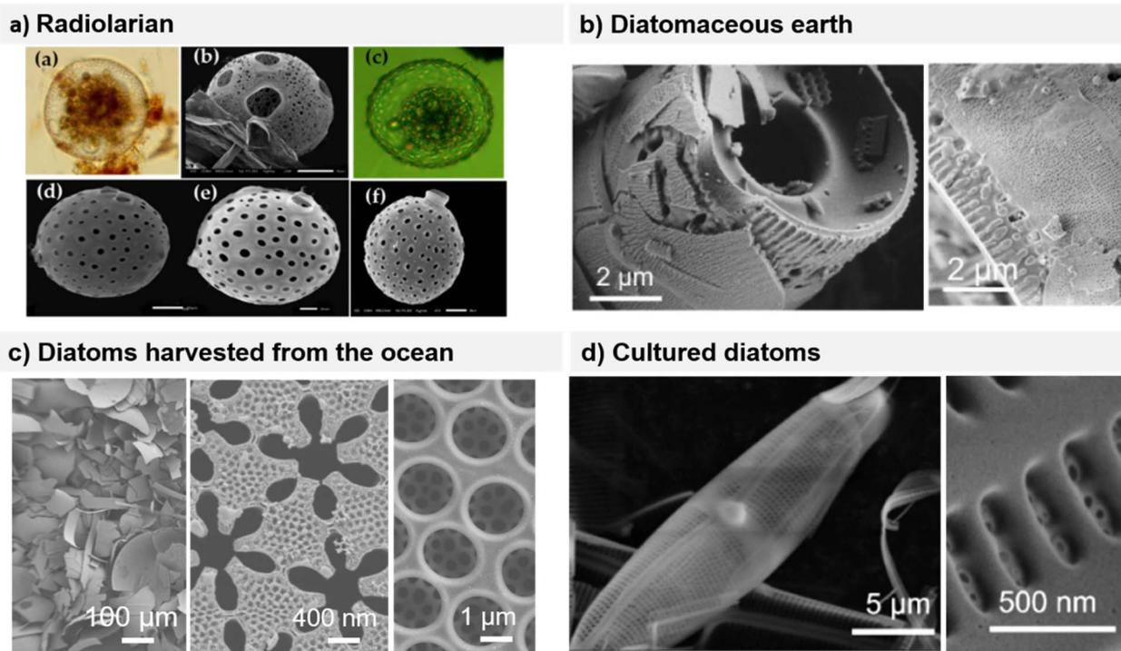
Fig. 2 SiO<sub>2</sub> exoskeletons from: (a) radiolarian, reproduced from ref. 32, (b) diatomaceous earth, reproduced from ref. 66, (c) diatoms harvested from the ocean, and (d) industrially cultured single-species diatom.<sup>66</sup>
