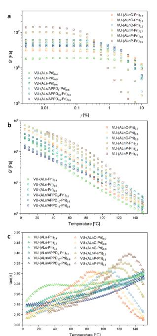
Fig. 4 DMA results of the lignin vitrimers based on lignosulfonate and enzymatic lignins ( $\omega = 6.28 \text{ rad s}^{-1}$ ,  $F_N = 1 \text{ N}$ ). (a) Amplitude-sweep measurement results of the tested lignin vitrimers (T = 110 °C). (b and c) Temperature-sweep measurements of the lignin vitrimers (T = 150 – 0 °C,  $\gamma = 0.01\%$ ), (b) storage modulus G', (c) loss factor  $\tan(\delta)$ .
