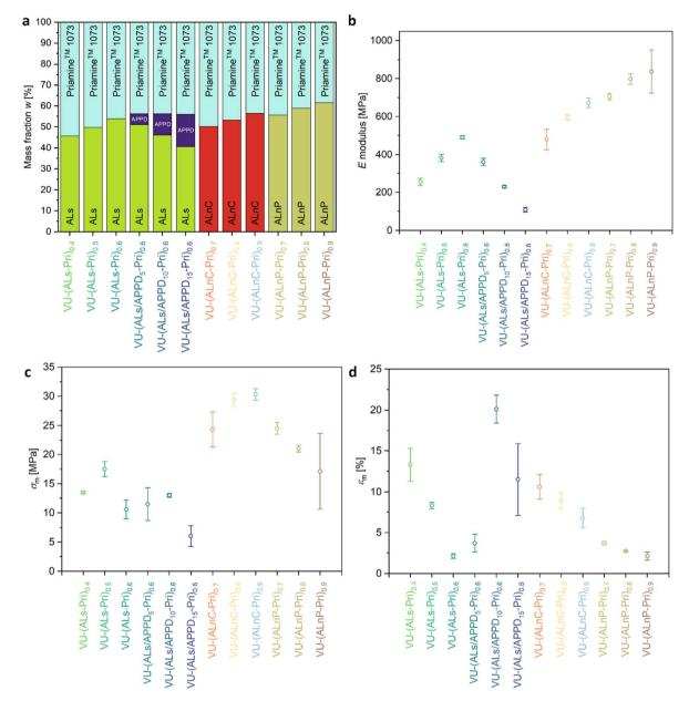
Fig. 3 (a) Mass fractions of the used building blocks of the lignin vitrimers with the acetoacetylated lignin species ALs, ALnC, and ALnP, respectively, the linear difunctional APPD, and the amount of Priamine  $^{\text{TM}}$  1073. (b-d) Tensile test data of the lignin vitrimers ( $T = 23 \, ^{\circ}\text{C}$ ), (b) tensile modulus (E), (c) tensile strengths ( $\sigma_{\rm m}$ ), (d) elongation at ultimate stress ( $\varepsilon_{\rm m}$ )
