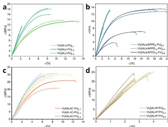
Fig. 2 Stress-strain curves ( $T = 23\text{ }^{\circ}\text{C}$ ) of the lignin vitrimer materials derived from ALs (a and b), ALnC (c), and ALnP (d). The materials range from softer films to more rigid ones, showing averaged elastic moduli ( $E$ ) in the range of 108 MPa up to 837 MPa, tensile strengths ( $\sigma_m$ ) of 6.0 MPa up to 30.3 MPa, and elongations at an ultimate stress ( $\varepsilon_m$ ) of 2.1% to 20.1%.
