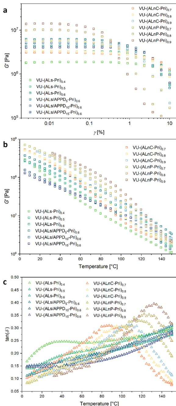
Fig. 4 DMA results of the lignin vitrimers based on lignosulfonate and enzymatic lignins ( $\omega = 6.28 \text{ rad s}^{-1}$ ,  $F_N = 1 \text{ N}$ ). (a) Amplitude-sweep measurement results of the tested lignin vitrimers ( $T = 110$  °C). (b) and (c) Temperature-sweep measurements of the lignin vitrimers ( $T = 150$ – $0$  °C,  $\gamma = 0.01\%$ ), (b) storage modulus  $G'$ , (c) loss factor  $\tan(\delta)$ .
