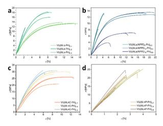
Fig. 2 Stress-strain curves (T = 23 °C) of the lignin vitrimer materials derived from ALs (a and b), ALnC (c), and ALnP (d). The materials range from softer films to more rigid ones, showing averaged elastic moduli (E) in the range of 108 MPa up to 837 MPa, tensile strengths ( $\sigma_{\rm m}$ ) of 6.0 MPa up to 30.3 MPa, and elongations at an ultimate stress ( $\varepsilon_m$ ) of 2.1% to 20.1%.
