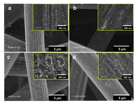
Fig. 1 SEM images of GDE-Pd/NiO $_x$  (before and after thermal treatment) deposited on a GDE (3  $\times$  3 cm $^2$ ) at different thicknesses: (a) GDE-Pd/NiO250, (b) GDE-Pd/NiO250-TT, (c) GDE-Pd/NiO1000, and (d) GDE-Pd/NiO1000-TT.
