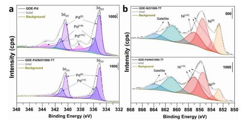
Fig. 3 High-resolution XPS spectra of the GDE-Pd/NiOX material: (a) Pd 3d XPS spectra of GDE-Pd (top) and GDE-Pd/NiO1000-TT (bottom), and (b) Ni 2p XPS spectra of GDE-NiO1000-TT (top) and GDE-Pd/NiO1000-TT (bottom).
