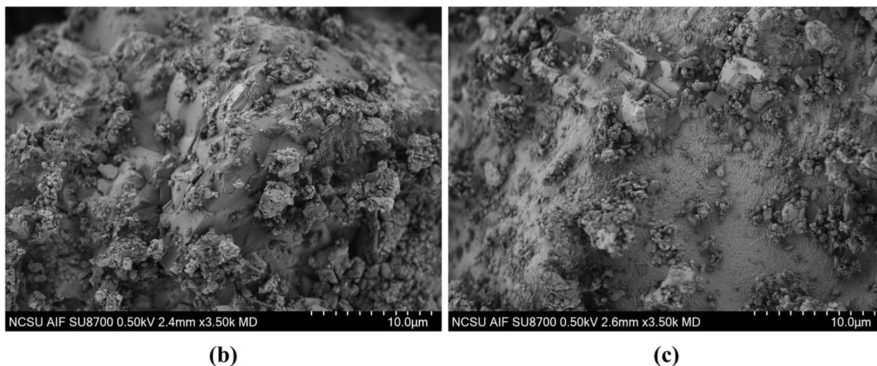
Fig. 8 Comparison of fresh and spent (after 100 cycles between 510 °C/20% O<sub>2</sub>-660 °C/Ar) LSF1:LiF-NaF-CaF<sub>2</sub> (0.4 : 0.6). (a) XRD patterns and SEM images of (b) after sintering, which corresponds to the morphology of composite material after 1 cycle (c) after 100 cycles.
