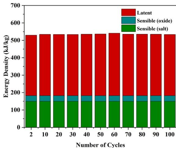
Fig. 7 TGA-DSC measurements for LSF1:LiF-NaF-CaF<sub>2</sub> with the weight ratio of 0.4:0.6 at 510 °C/20% O<sub>2</sub>-660 °C/Ar during 100 cycles. (a) Overall energy density (kJ kg<sup>-1</sup>). Latent heat is the measured melting enthalpy from DSC. Sensible heat is based on estimated heat capacities through additive principle using NIST database.<sup>62</sup>
