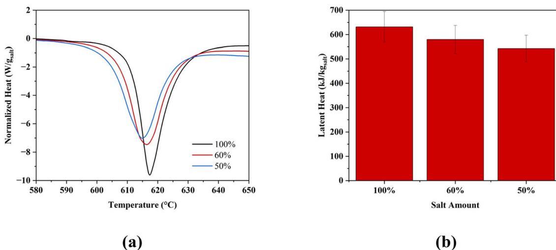
**Fig. 6** Comparison of LSF1:LiF–NaF–CaF<sub>2</sub> at various salt amounts. (a) Normalized heat flows ( $\text{W g}_{\text{salt}}^{-1}$ ) and (b) latent heats ( $\text{kJ kg}_{\text{salt}}^{-1}$ )
