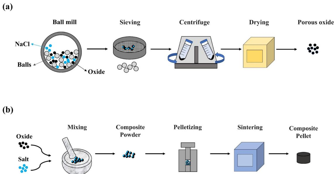
Fig. 1 Schematic representation of material preparation (a) salt-grinding method for the formation of porous oxide (b) composite material preparation *small portion of the composite particles were used for TGA-DSC tests, while the rest was prepared for the XRD analysis.*
