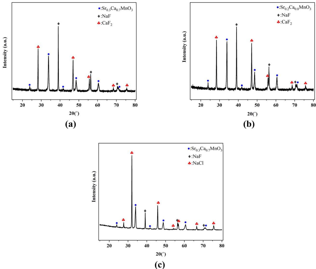
Fig. 2 XRD patterns of composite materials with Ca-based perovskites (a) SCFM1:NaF–CaF<sub>2</sub>, (b) SCFM2:NaF–CaF<sub>2</sub> and (c) SCFM2:NaF–NaCl.
