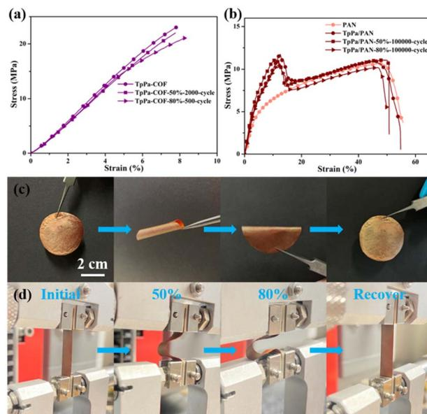
Fig. 4 Stress–strain curves of self-standing TpPa-COF, TpPa-50%-2000-cycle, and TpPa-80%-500-cycle membranes (a). Stress–strain curves of PAN fiber, TpPa/PAN, TpPa/PAN-50%-100,000-cycle, TpPa/PAN-80%-100,000-cycle membranes (b). The test of self-standing TpPa membrane under bending and folding states (c), and the bending and recovery process under a compression rate of 50% and 80% (d).
