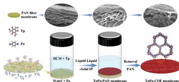
Fig. 1 Diagrammatic representation of the preparation process of TpPa/PAN and self-standing TpPa-COF membranes.
