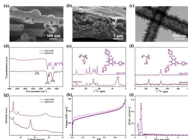
Fig. 3 Cross-sectional SEM pictures of self-standing membranes (a and b). TEM images of hollow TpPa fibers (c). FT-IR spectra (d), <sup>13</sup>C and <sup>15</sup>N CP MAS solid-state NMR spectra (e and f), and PXRD patterns (g) of TpPa/PAN membrane and self-standing TpPa-COF membrane. N<sub>2</sub> adsorption-desorption isotherms (h) and pore size distribution (i) of self-standing TpPa-COF membrane.
