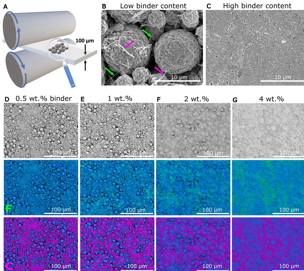
**Fig. 1** (A) Schematic of the electrode calendaring process. (B and C) SEM micrographs of NMC electrodes containing 0.5 and 4 wt% PTFE, respectively. (D–G) (Top) SEM micrographs of NMC electrodes containing 0.5, 1, 2 and 4 wt% PTFE, respectively. Middle: corresponding EDX maps showing the active material (Ni–O signal) and binder (F signal) in blue and green, respectively. (Bottom) EDX maps showing the active material (Ni–O signal) and carbon additive (C signal) in blue and pink, respectively.
