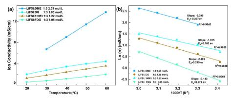
Fig. 2 The (a) ion conductivity of probed electrolytes (for the LiFSI: DME 1: 3 (molar: molar) electrolyte, the ion conductivity at 20 °C is missing because the electrolyte got frozen under 20 °C, as shown in Fig. S4†); (b) activation energies obtained from the Arrhenius equation for the tested electrolyte systems.
