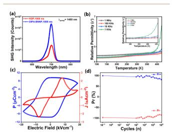
Fig. 2 (a) The spectra of the SHG response of DIPA · BNPP with respect to the reference KDP. (b)Temperature-dependent relative permittivity of DIPA·BNPP. (c) The P-E hysteresis loop and leakage current density plot of DIPA·BNPP. (d) Fatigue profile data of DIPA·BNPP up to 10<sup>6</sup> cycles.
