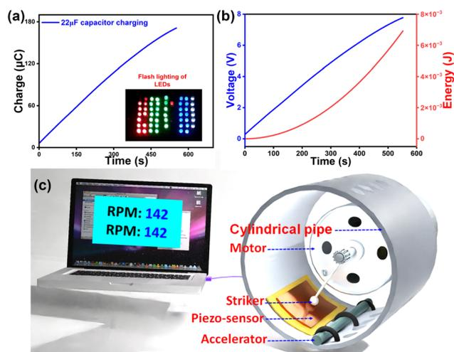
Fig. 5 (a) The graph of charge storage by using the 22  $\mu\text{F}$  capacitor, and the inset image shows the demonstration of flash lighting of 53 LEDs. (b) Voltage and energy vs. time profile during charging of a 22  $\mu\text{F}$  capacitor. (c) Schematic representation of an RPM sensor based on **DIPA·BNPP**.
