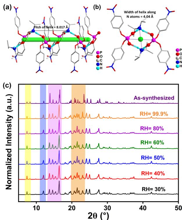
Fig. 1 (a) Formation of a 1D-helical chain structure in **DIPA·BNPP** mediated by hydrogen bonding interactions along the  $b$ -axis. (b) Top-view of the helical assembly along the  $c$ -axis. (c) Humidity dependent PXRD profiles of **DIPA·BNPP** showing its high moisture stability.
