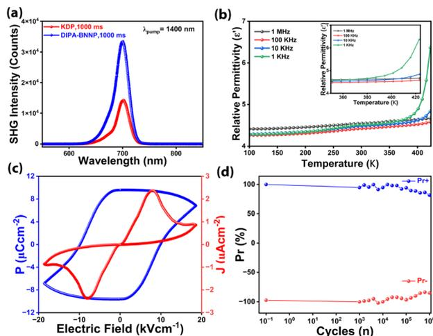
Fig. 2 (a) The spectra of the SHG response of **DIPA·BNPP** with respect to the reference KDP. (b) Temperature-dependent relative permittivity of **DIPA·BNPP**. (c) The  $P$ – $E$  hysteresis loop and leakage current density plot of **DIPA·BNPP**. (d) Fatigue profile data of **DIPA·BNPP** up to  $10^6$  cycles.
