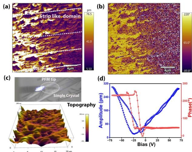
Fig. 3 PFM analysis of  $\text{DIPA} \cdot \text{BNPP}$  showing (a) its vertical amplitude and (b) phase images. (c) The visualization of a single crystal of  $\text{DIPA} \cdot \text{BNPP}$  on the drop-cast thin film along with the PFM tip and its 3D-topography image. (d) The SS-PFM spectroscopy derived amplitude-butterfly and phase-hysteresis loops as a function of voltage bias at a single point on the  $\text{DIPA} \cdot \text{BNPP}$  film substrate.
