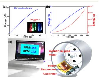
Fig. 5 (a) The graph of charge storage by using the 22 μF capacitor, and the inset image shows the demonstration of flash lighting of 53 LEDs. (b) Voltage and energy vs. time profile during charging of a 22  $\mu$ F capacitor. (c) Schematic representation of an RPM sensor based on DIPA · BNPP.
