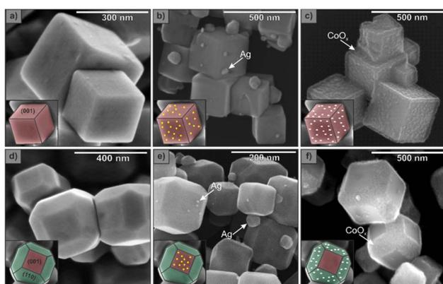
Fig. 4 The SEM images of the  $\text{SrTiO}_3$  cubes and rhombic dodecahedrons with photodeposited silver or cobalt(III) oxide. Cubic  $\text{SrTiO}_3$  crystals before photodeposition (a), loaded with Ag (b) and  $\text{Co}_2\text{O}_3$  (c). Rhombic dodecahedrons of  $\text{SrTiO}_3$  before photodeposition (d), loaded with Ag (e) and  $\text{Co}_2\text{O}_3$  (f).
