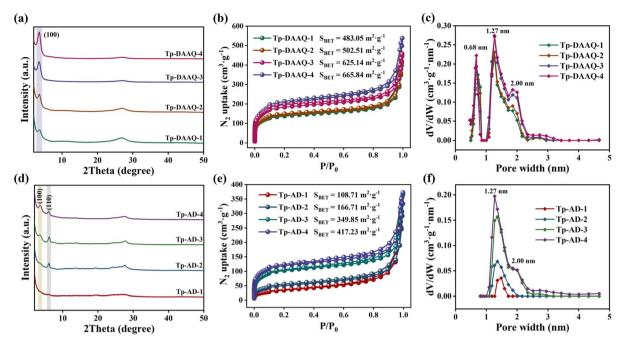
Fig. 2 (a) PXRD patterns, (b) N<sub>2</sub> adsorption-desorption isotherms and (c) pore size distributions of the defective DAAQ-COFs (Tp-DAAQ-1, Tp-DAAQ-2, Tp-DAAQ-3 and Tp-DAAQ-4). (d) PXRD patterns, (e) N<sub>2</sub> adsorption – desorption isotherms and (f) pore size distributions of the defective AD-COFs (Tp-AD-1, Tp-AD-2, Tp-AD-3 and Tp-AD-4).
