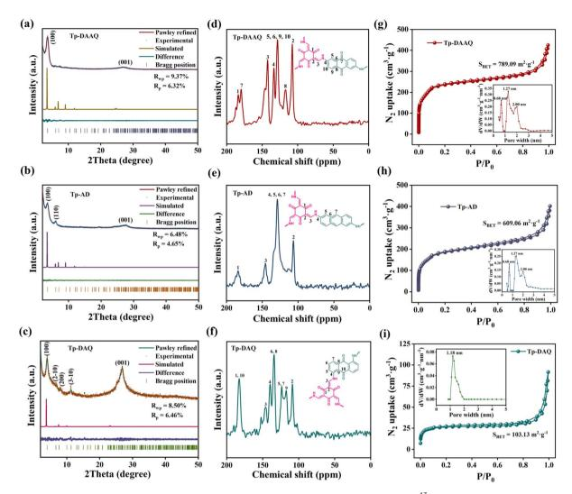
Fig. 1 Experimental and Pawley refined PXRD of (a) Tp-DAAQ, (b) Tp-AD and (c) Tp-DAQ. Solid-state <sup>13</sup>C NMR spectra of (d) Tp-DAAQ, (e) Tp-AD and (f) Tp-DAQ. N<sub>2</sub> adsorption—desorption isotherms and the corresponding pore size distributions (inset) of (g) Tp-DAAQ, (h) Tp-AD and (i) Tp-DAQ.
