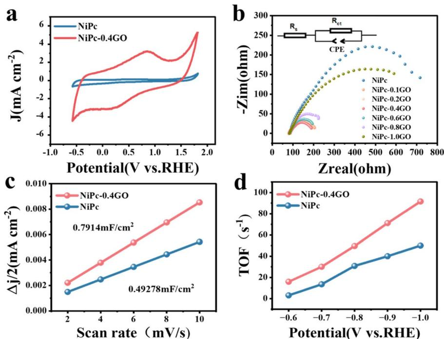
Fig. 6 (a) Cyclic voltammograms of NiPc and NiPc-0.4GO. (b) EIS data for different NiPc-GO composites and NiPc. (c) Linear plots of the  $1/2$  current density difference versus scan rate for NiPc-0.4GO and NiPc. (d) TOF plots of NiPc-0.4GO and NiPc at different potentials.
