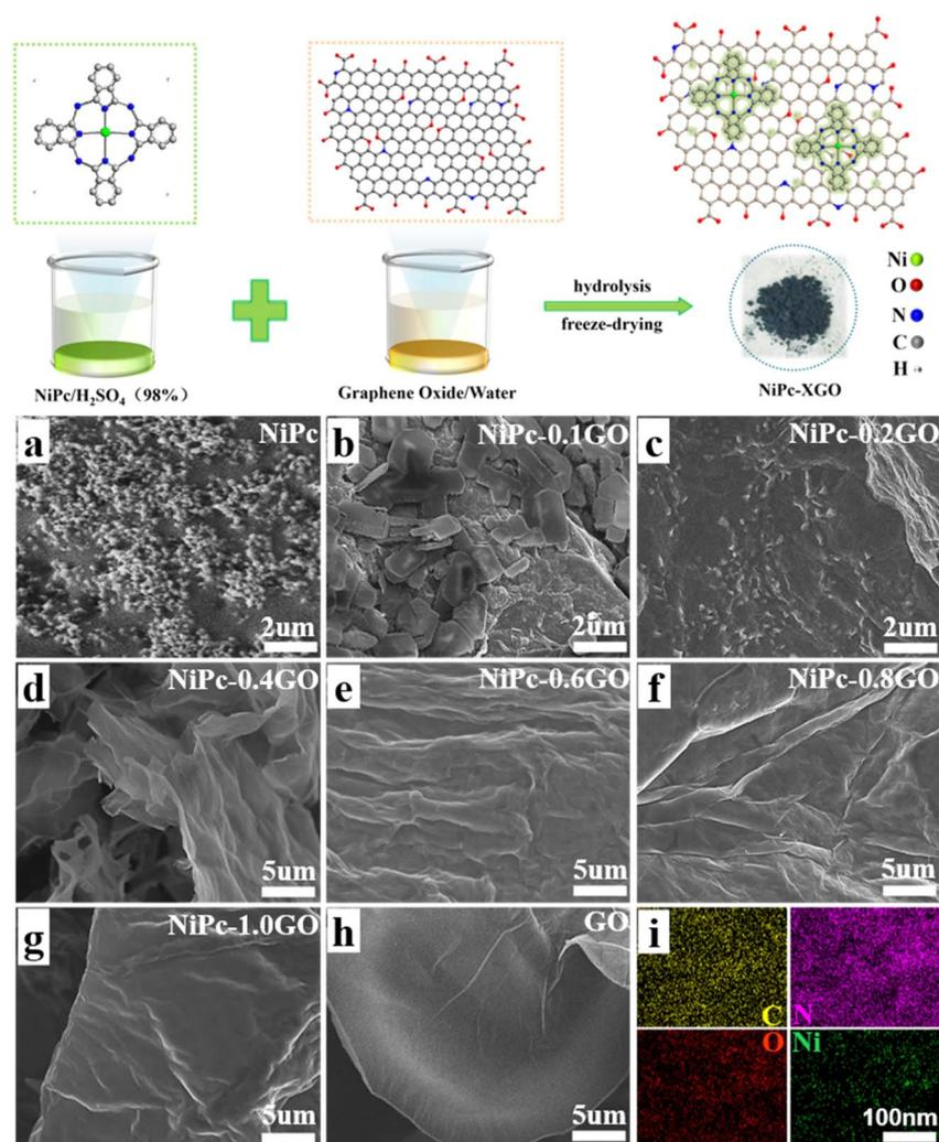
**Fig. 1** Schematic illustration of the synthesis of NiPc/GO composites. SEM images of (a) NiPc, (b) NiPc–0.1GO, (c) NiPc–0.2GO, (d) NiPc–0.4GO, (e) NiPc–0.6GO, (f) NiPc–0.8GO, (g) NiPc–1.0GO, and (h) GO. (i) Elemental mappings of C, N, O, and Ni atoms.
