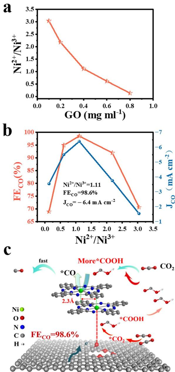
Fig. 8 (a) The variation of  $\text{FE}_{\text{CO}}/J_{\text{CO}}$  with the  $\text{Ni}^{2+}/\text{Ni}^{3+}$  ratio at a potential of  $-0.9 \text{ V}_{\text{RHE}}$ . (b) The linear correlation between the mass concentration of GO and the  $\text{Ni}^{3+}/\text{Ni}^{2+}$  ratio in NiPc-0.1GO, NiPc-0.2GO, NiPc-0.4GO, NiPc-0.6GO, NiPc-0.8GO, and NiPc-1.0GO. (c) Catalytic mechanism of NiPc-0.4GO in CO<sub>2</sub> reduction.
