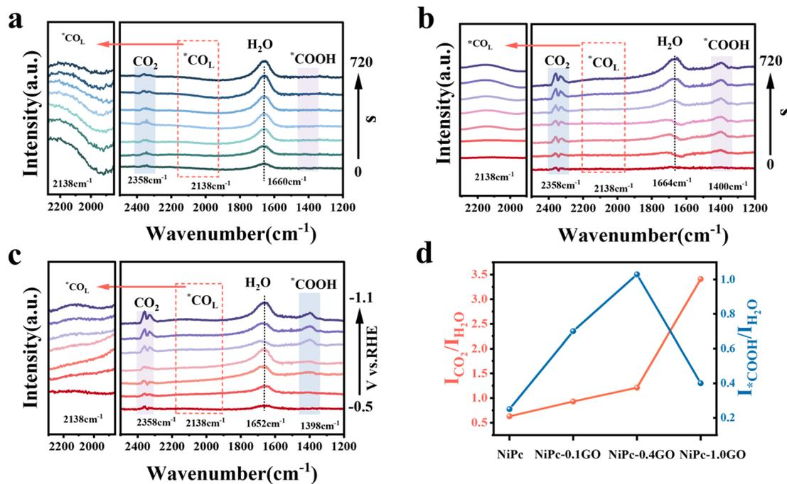
Fig. 7 Time-dependent *in situ* DRIFTS spectra of (a) NiPc and (b) NiPc-0.4GO samples for CO<sub>2</sub>RR at -0.9 V vs. RHE. (c) *In situ* DRIFTS spectra of NiPc-0.4GO at different work potentials. (d) Change in the  $I_{\text{CO}_2}/I_{\text{H}_2\text{O}}$  and  $I_{*\text{COOH}}/I_{\text{H}_2\text{O}}$  ratios in *in situ* DRIFTS spectra of NiPc, NiPc-0.1GO, NiPc-0.4GO, and NiPc-1.0GO at -0.9 V vs. RHE.
