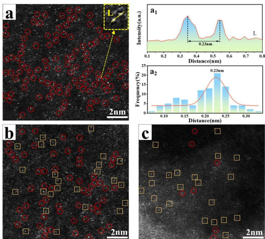
Fig. 2 HADDF-STEM images of (a) NiPc-0.4GO, (b) NiPc-0.6GO, and (c) NiPc-0.8GO samples. (a<sub>1</sub>) Intensity profiles along the arrows and (a<sub>2</sub>) Ni-Ni distance distribution of NiPc-0.4GO.
