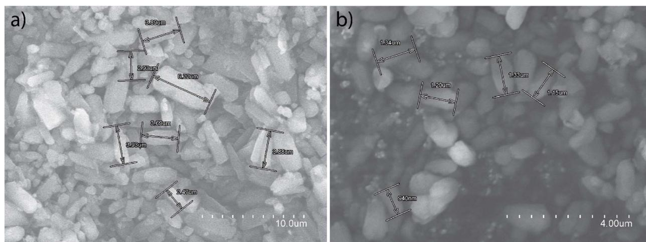
**Fig. 2** SEM images of a polycrystalline sample of **3** at two different magnifications (a and b) with selected sizes marked.
