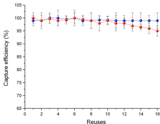
Fig. 3 Reuses of MOF 3 (blue) and activated carbon (red) for the removal (%) of fentanyl using a  $20 \mu\text{g L}^{-1}$  aqueous solution. Error bars of three independent replicate measurements are included.
