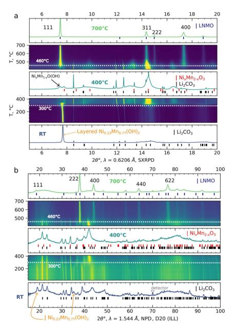
Fig. 1 In situ T-controlled SXRPD (a) and NPD data (b) of the mixture of  $Li_2CO_3$  and  $Ni_{0.23}Mn_{0.77}(OH)_2$  collected at room temperature (bottom), at 400 °C (middle) and at 700 °C (top). Contour plots represent the evolution of SXRPD patterns from room temperature to 400 °C, and from 400 °C to 700 °C.
