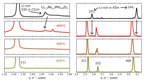
Fig. 8 Comparison of the SXRPD pattern of the Li-rich  $\text{Li}_{12}\text{Ni}_{0.2}\text{Mn}_{0.6}\text{O}_2$  oxide with the SXRPD patterns of the selected quenched samples. The ranges are chosen to highlight the superstructure reflections of the Li-rich layered oxide (left) and its main reflections (right).
