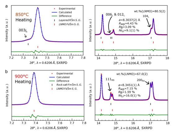
Fig. 4 Experimental points, as well as calculated and difference profiles obtained after the Rietveld refinement of the SXRPD patterns collected *in situ* for the 1:4 molar mixture of  $Li_2CO_3$  and  $Ni_{0.23}Mn_{0.77}(OH)_2$ : at 850 °C (a) and at 900 °C (b).  $2\theta$  ranges are selected to highlight reflections of the layered oxide and rock salt impurities, respectively.
