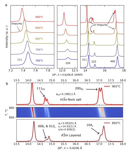
Fig. 3 Selected  $2\theta$  ranges of in situ SXRPD patterns collected for the 1:4 molar mixture of  $\text{Li}_2\text{CO}_3$  and  $\text{Ni}_{0.23}\text{Mn}_{0.77}(\text{OH})_2$  at given temperatures (a). Contour plot representing evolution of the SXRPD patterns from 850 °C to 903 °C during the in situ experiment (b).
