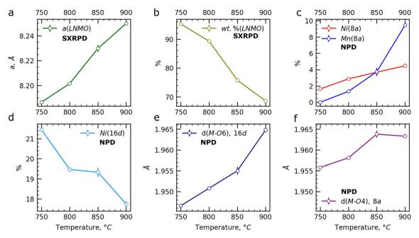
Fig. 7 Lattice parameter (a), weight fraction (b), Ni and Mn content at the Li 8a sites (c), Ni content at the M 16d sites, the Mn content being the complement of Ni in the 16d sites (d), interatomic distances at the 16d (e) and 8a (f) sites in the LNMO spinel phase after the Rietveld refinement of the SXRPD and NPD patterns of the q750 °C, q800 °C, q850 °C and q900 °C samples. The data source of each refined parameter is indicated in bold on the corresponding graph.
