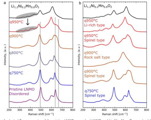
Fig. 9 Comparison of selected Raman spectra of the pristine LNMO, quenched LNMO and  $Li_{1.2}Ni_{0.2}Mn_{0.6}O_2$  samples (a). Comparison of the different Raman spectra that can be obtained for the q900 °C and q950 °C samples, collected from different particles, with the spectra of the q750 °C and  $Li_{1.2}Ni_{0.2}Mn_{0.6}O_2$  samples (b).
